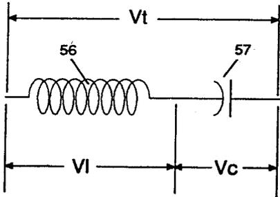
FIGURE 3-28: LC CIRCUIT SCHEMATIC
