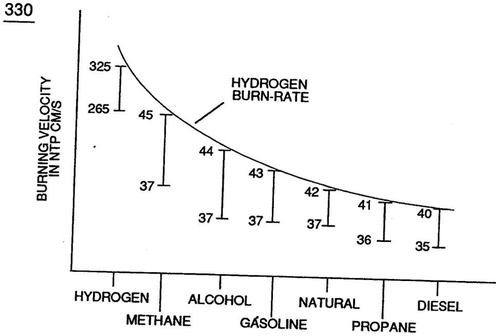
FIGURE 3-37: HYDROGEN BURN-RATE
