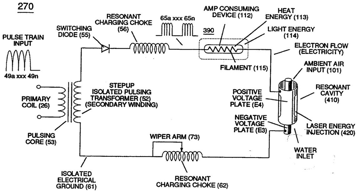
FIGURE 3-34: ELECTRON EXTRACTION CIRCUIT
