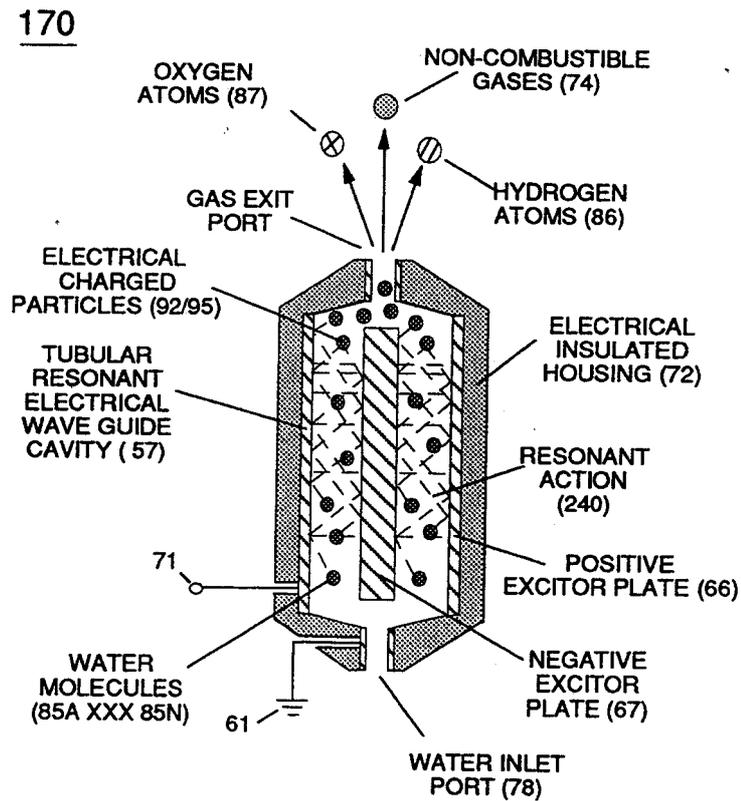
FIGURE 3-25: RESONANT CAVITY
