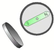
Using a compass to identify the pole of a magnet. The Pembina Institute
