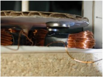
The magnets should pass as close to the coils as possible. The Pembina Institute
