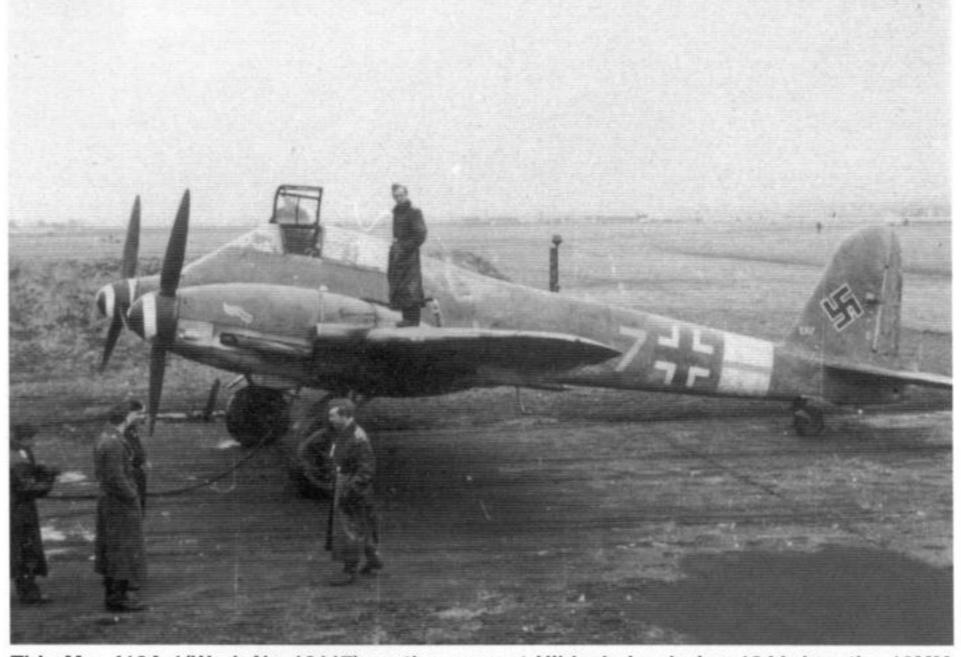
This Me 410A-1(Werk Nr. 10117) on the ramp at Hildesheim during 1944, has the 13MM gun barbettes and cockpit canopy radio mast deleted. The Yellow number, 7, and horizontal bar marking identify this aircraft as belonging to *II. Gruppe*. (Petrick)
