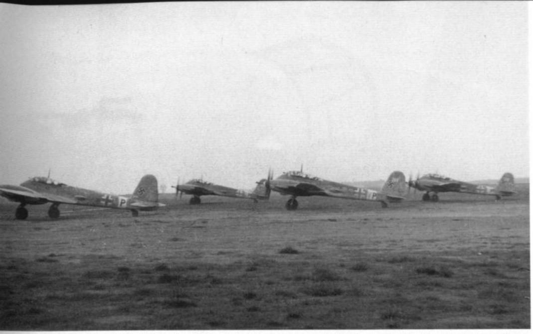
Four Me 410B-2/U-4s (3U+MP, 3U+CP, 3U+VP and 3U+LP) of 6./ZG 26 are starting their takeoff roll on another interception mission. The individual identification letter on each aircraft was in red. Two of the aircraft carry three digits of the Werk Number on the vertical stabilizer in White. (Petrick)
