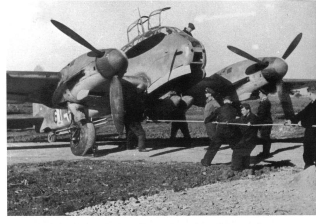
The gun turret cover has been removed so that armament crews can load belted 13mm ammunition into the starboard MG 131 gun turret on this Me 210A-1, while other crewmen prepare to load the bomb bay. Other mechanics are servicing the cockpit, making sure that all is in readiness for the aircraft's next mission. (Petrick)
