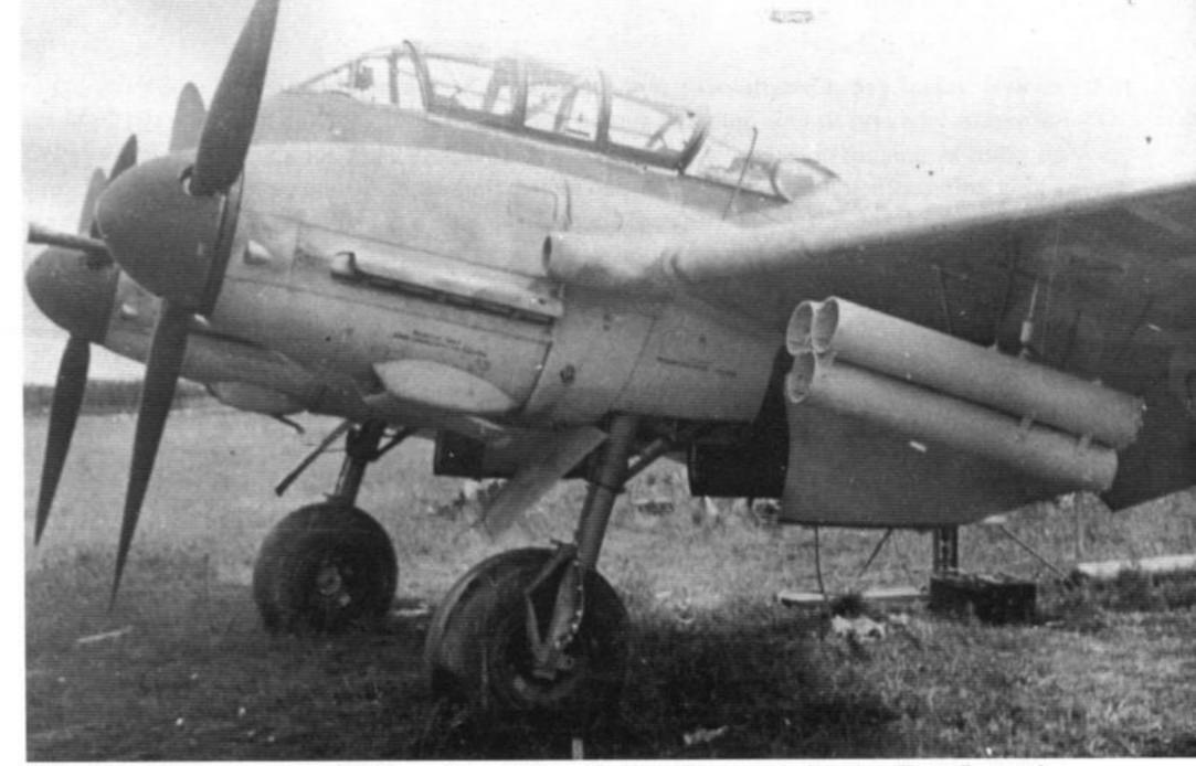
This Me 210 was modified with a 40mm 39M anti-aircraft cannon for the *Zerstörer* role. Additionally, ZO+03 also carried three 150mm rocket tubes under each outer wing panel. The aircraft was based at Varpalota during October of 1944. It was decided to modify thirty aircraft to this configuration, but only four were actually finished. (Punka)
