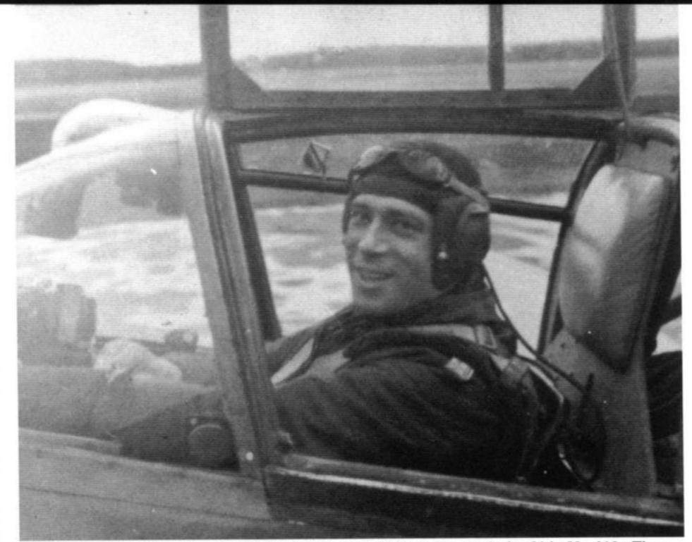
Oberleutnant Jenne, Gruppenkommander of I./ZG 26 in the cockpit of his Me 410. The front armored glass panel has been removed and the Revi gunsight is visible under the small bubble in the windshield. There is a small mirror mounted on the canopy framing (just to the left of the pilot's head). (Wiesinger via Wenko)
