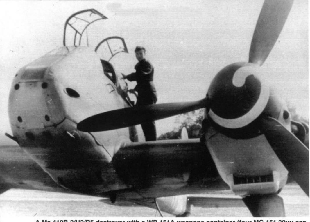
A Me 410B-2/U2/R5 destroyer with a WB 151A weapons container (four MG 151 20mm cannons) in the bomb bay. This aircraft has also been modified to carry an additional two 7.9mm MG 17s in the nose directly above the weapons bay. The port cabin air intake is closed. (Dressel)
