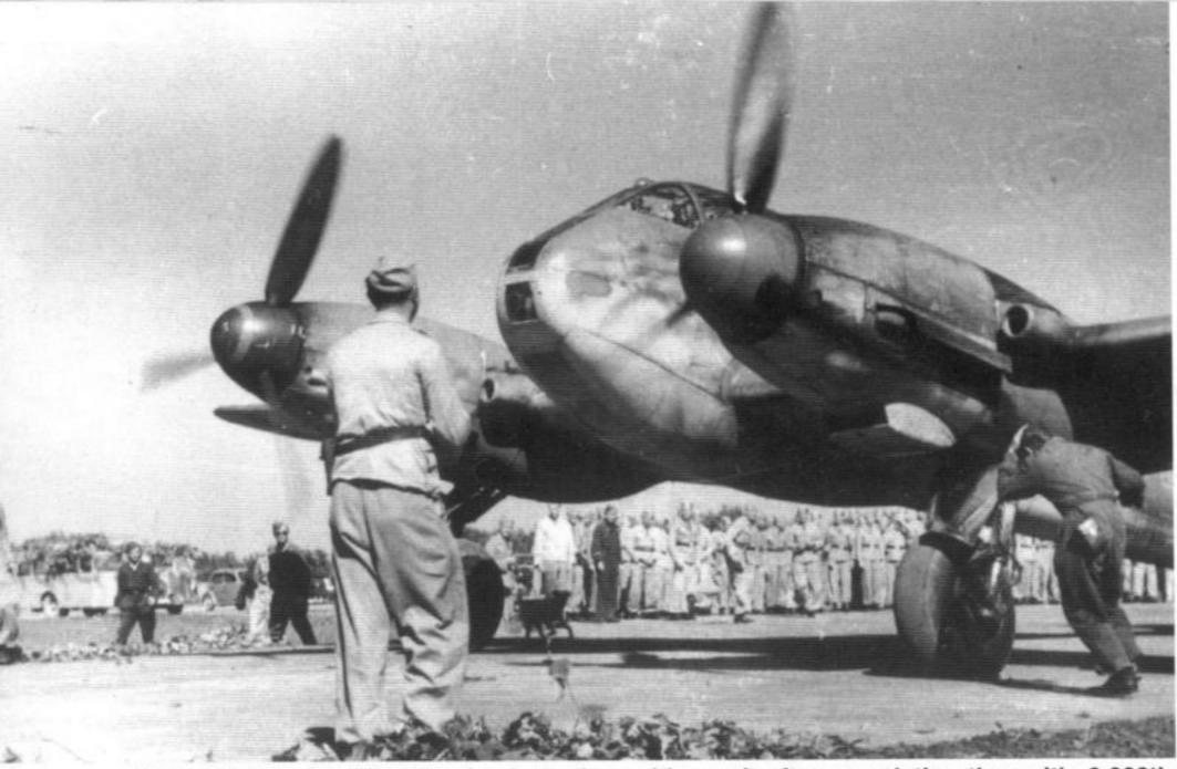
A Me 410A-3 of 2./(F)122 taxies in to the waiting unit after completing the unit's 3,000th sortie. The Me 410A-3 had all forward firing armament removed and the ports faired over. The windows in the underside of the nose were camera ports. (Smithsonian)
