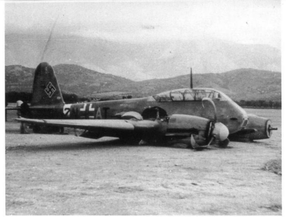
This Me 210A-1 (2N+AT, Werk Nr. 039) made a forced landing at Castelli on 8 November 1942. The aircraft had the A of the radio code in Yellow and the Werk Number on the vertical fin was in White. Crewmen have already begun to remove panels from the aircraft. (Petrick)
