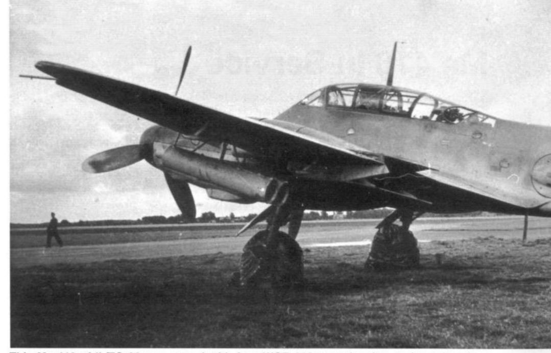
This Me 410 of II./ZG 26 was armed with four WGR 210mm underwing rocket tubes (two under each outer wing panel). The Holzschuh unit insignia is just visible on the engine cowling just above the rocket tube. (Petrick)
