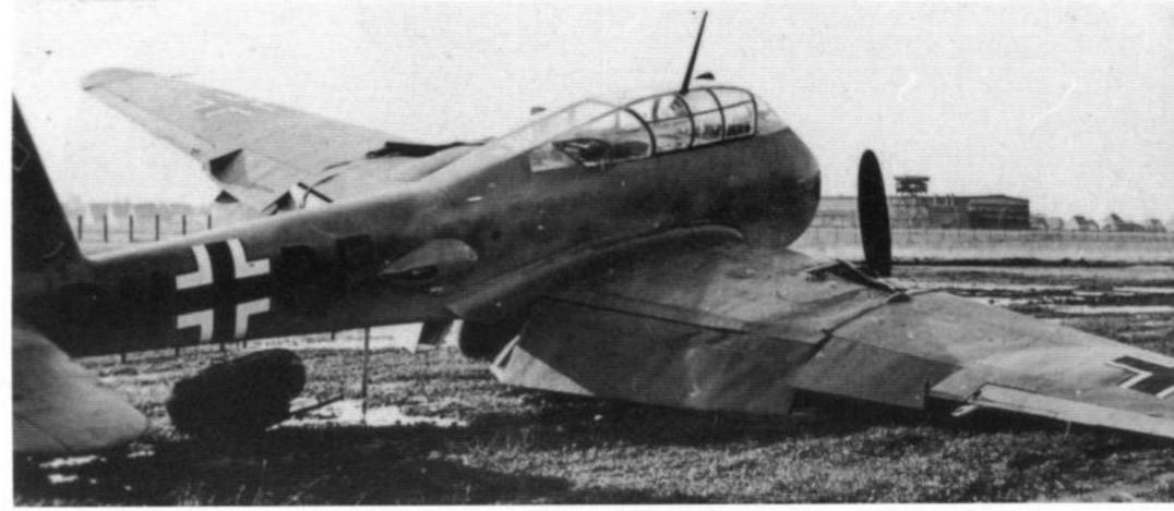
This Me 210A-1 (PN+PF, Werk Nr.107) had the starboard landing gear leg fail on landing. The crew of two was housed under a bubble type canopy, with the radio-operator/gunner facing the rear. (Mohr)
