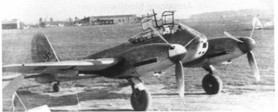
A Messerschmitt Me 410B-1/U2 (Werk Nr. 410096) of a training unit in Braunschweig-Waggum. This particular aircraft has no exhaust shrouds over the engine exhaust ports. The Me 410B-1/U-2 was armed with 13mm guns replacing the 7.9mm machine guns and an additional pair of 20mm cannons in the bomb bay. (Wiesinger via Obst. E. Peter)
