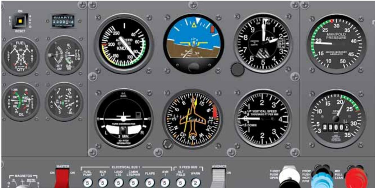
Figure 11-8. Vacuum Failure.
