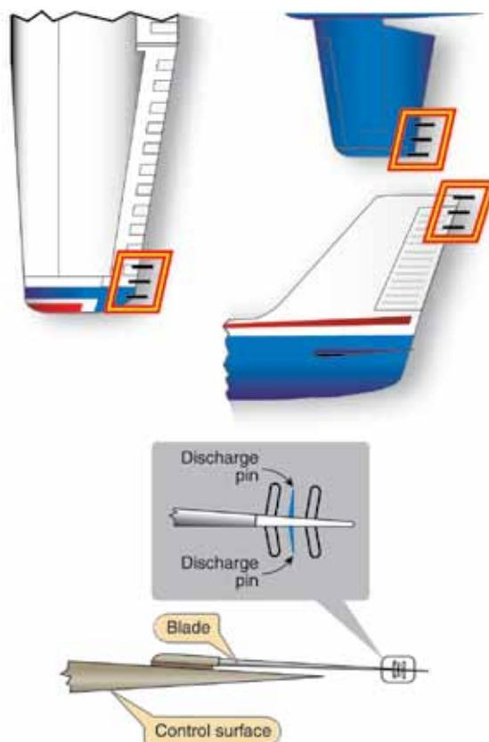
**Figure 11-2.** *One example of a static wick installed on aircraft control surface to bleed off static charges built up during flight. This will prevent static buildup and St. Elmo's fire by allowing the static electricity to dissipate harmlessly.*
