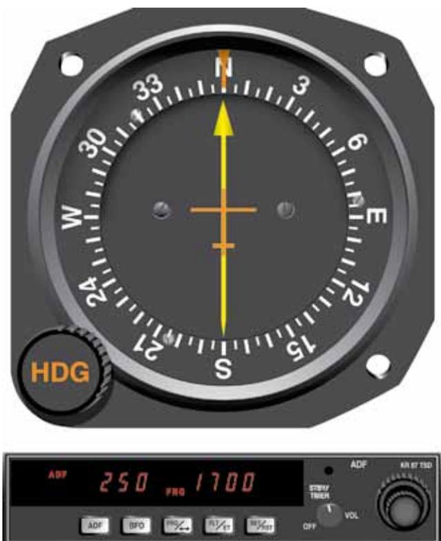
Figure 7-2. ADF Indicator Instrument and Receiver.
