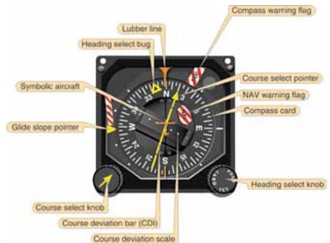
**Figure 7-13.** A Typical Horizontal Situation Indicator (HSI).
