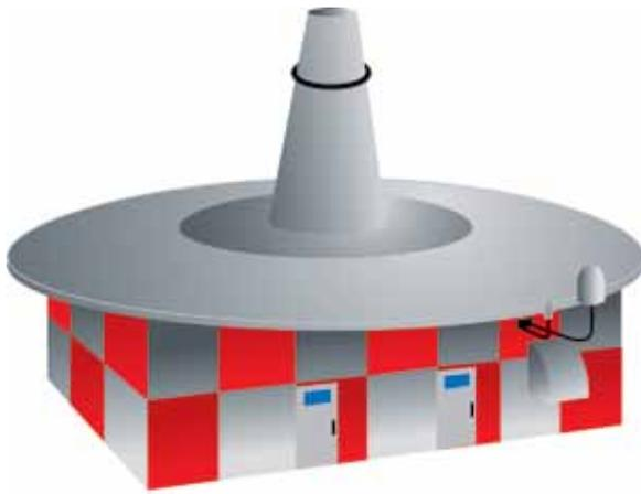
**Figure 7-11.** VOR Transmitter (Ground Station).
