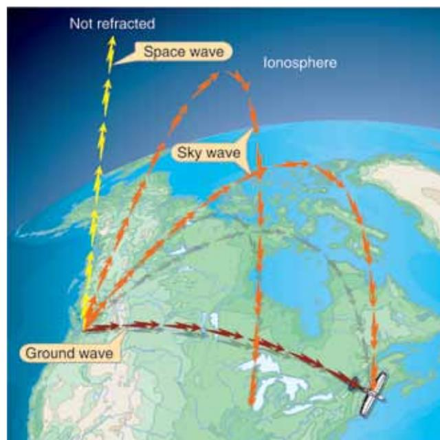
Figure 7-1. Ground, Space, and Sky Wave Propagation.
