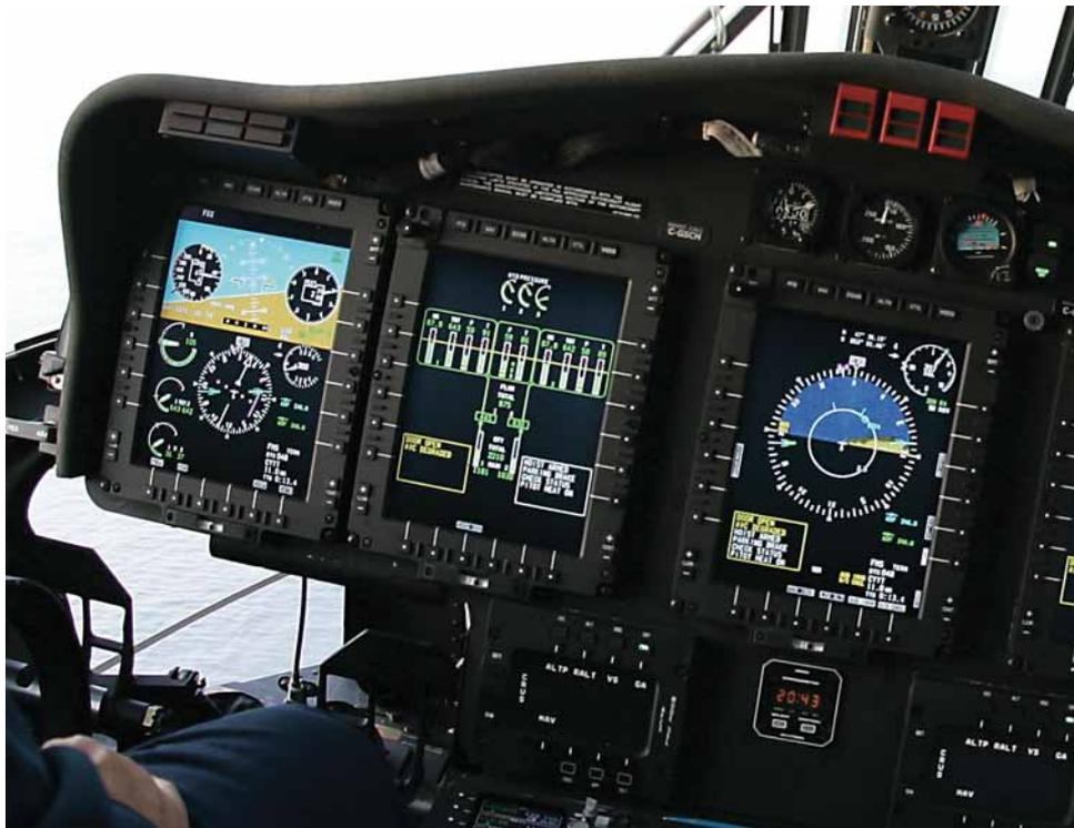
Figure 6-20. MFD Display of Aircraft Systems.
