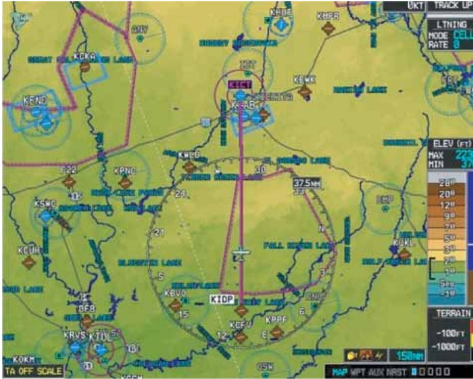
Figure 6-19. MFD Display of a Moving Map.
