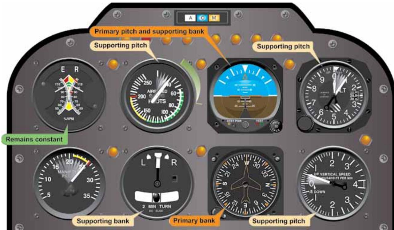
Figure 6-16. Flight Instrument Indications During an Instrument Takeoff.
