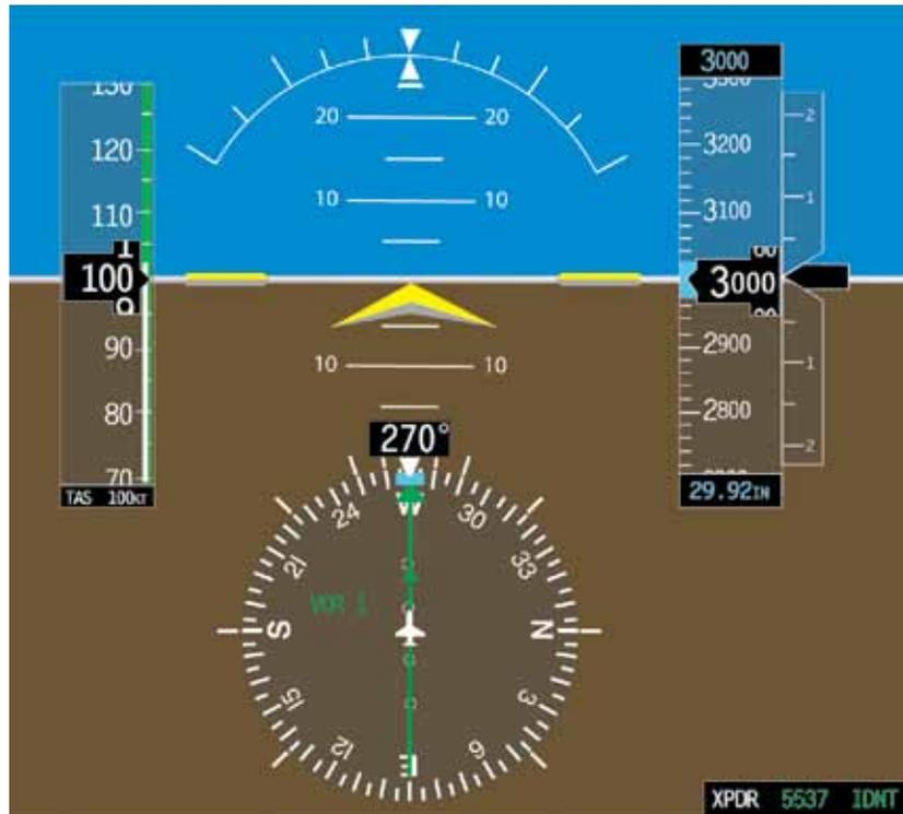
Figure 6-17. PFD Indications During Straight-and-Level Flight.
