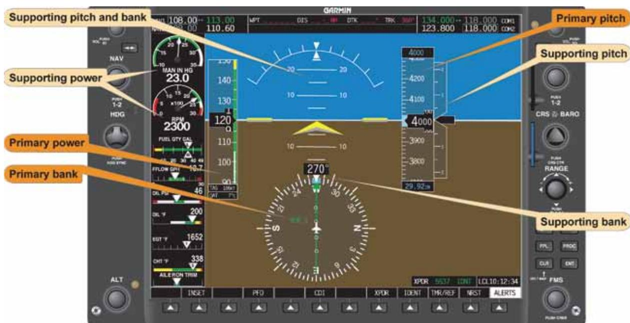
**Figure 5-57.** *Straight-and-Level Flight (Normal Cruising Speed).*
