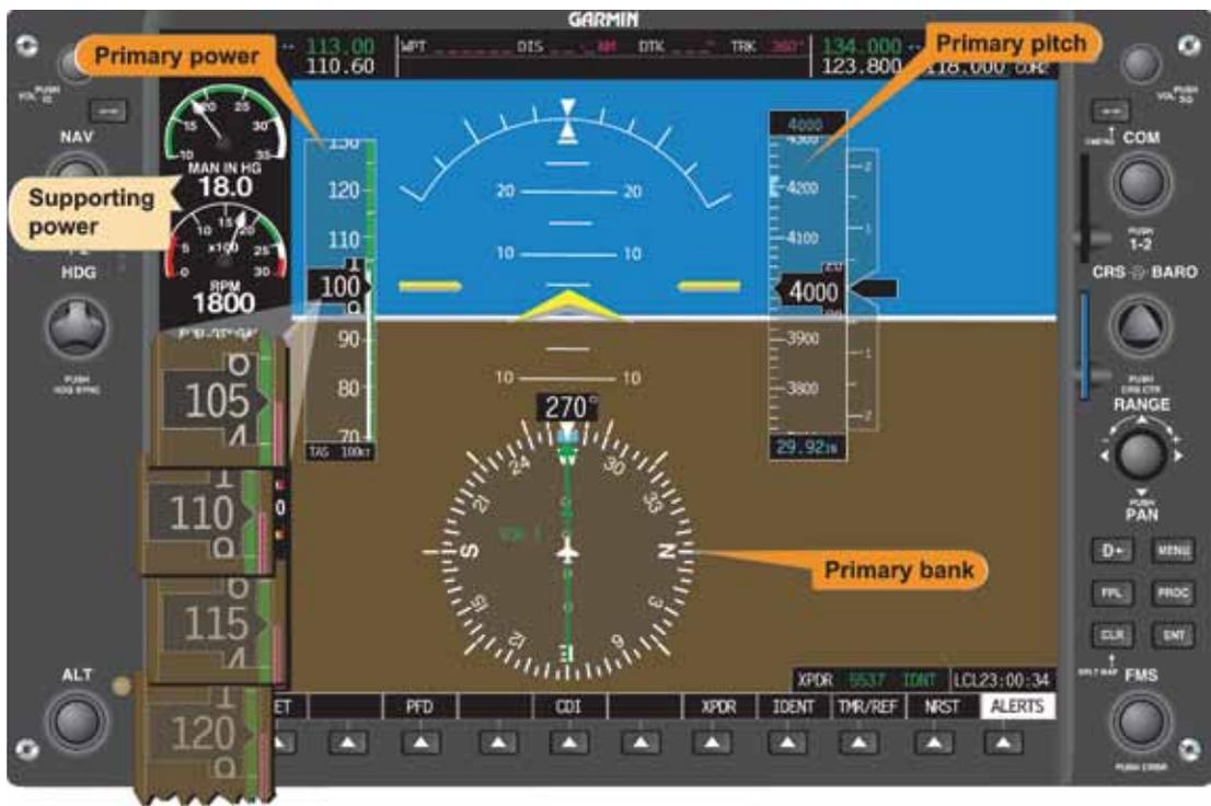
Figure 5-59. Straight-and-Level Flight (Reduced Airspeed Stabilized).
