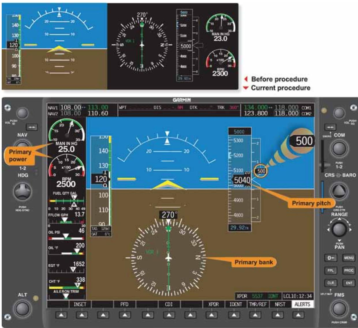
Figure 5-63. Constant Airspeed Climb From Cruise Airspeed.
