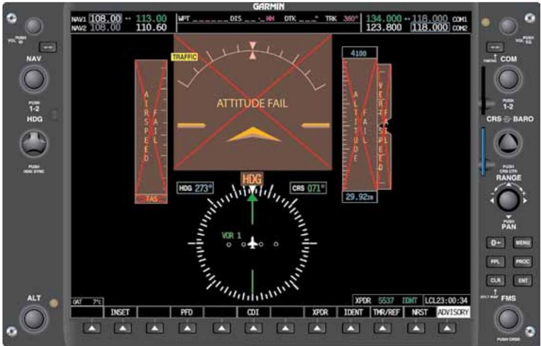
Figure 5-74. AHRS ADC Failure.
