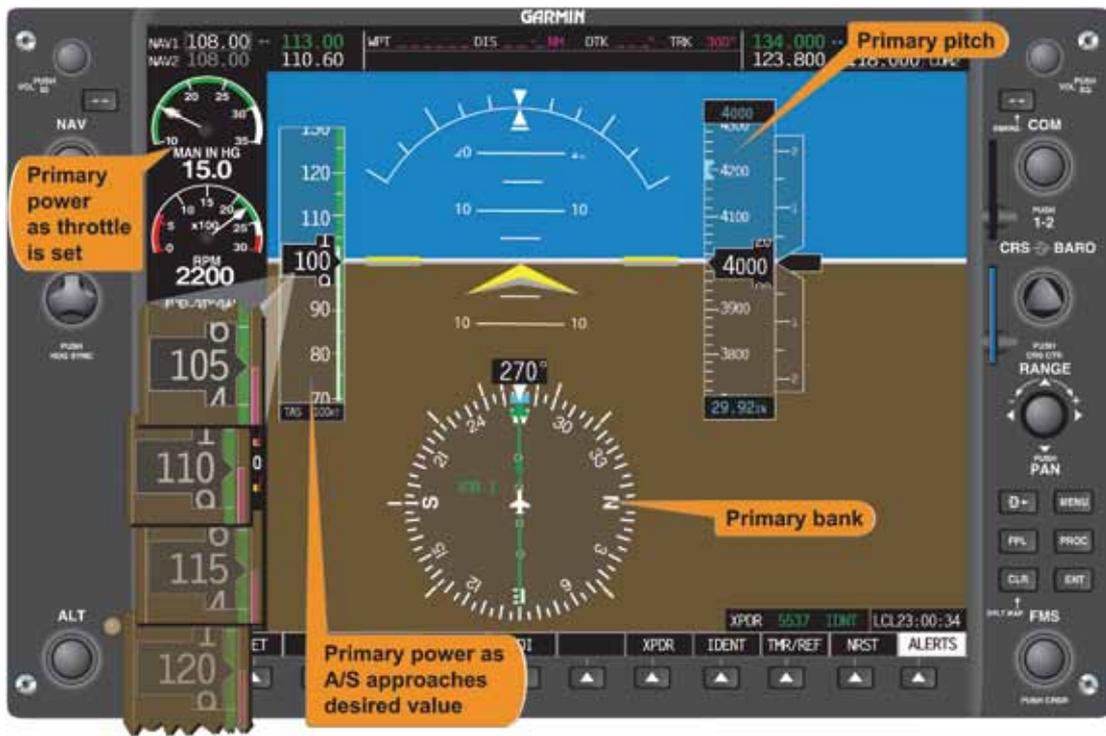
Figure 5-58. Straight-and-Level Flight (Airspeed Decreasing).
