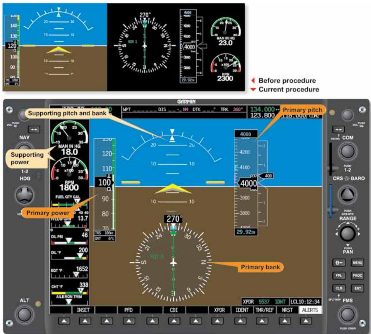
Figure 5-64. Constant-Airspeed Climb From Established Airspeed.
