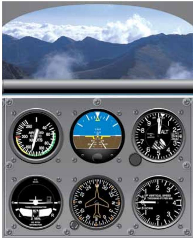
Figure 5-2. Pitch Attitude and Airspeed in Level Flight, Fast Cruise Speed.
