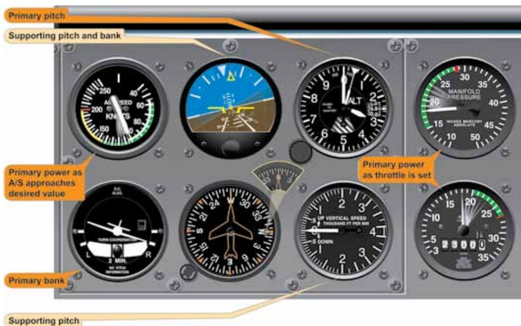
Figure 5-38. Change of Airspeed During Turn.
