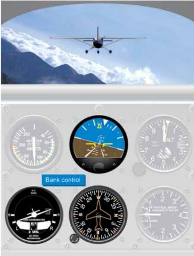
**Figure 5-16.** Instruments Used for Bank Control.
