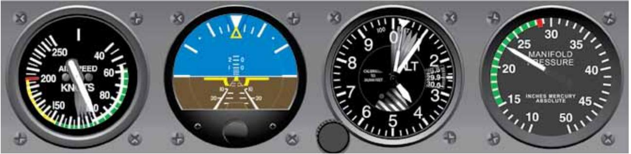
**Figure 5-20.** *Airspeed Low and Altitude High—Lower Pitch.*
