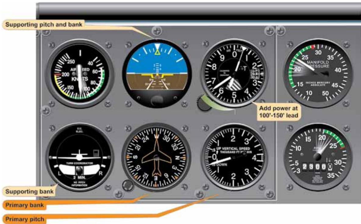
Figure 5-31. Level Off Airspeed Higher Than Descent Airspeed.
