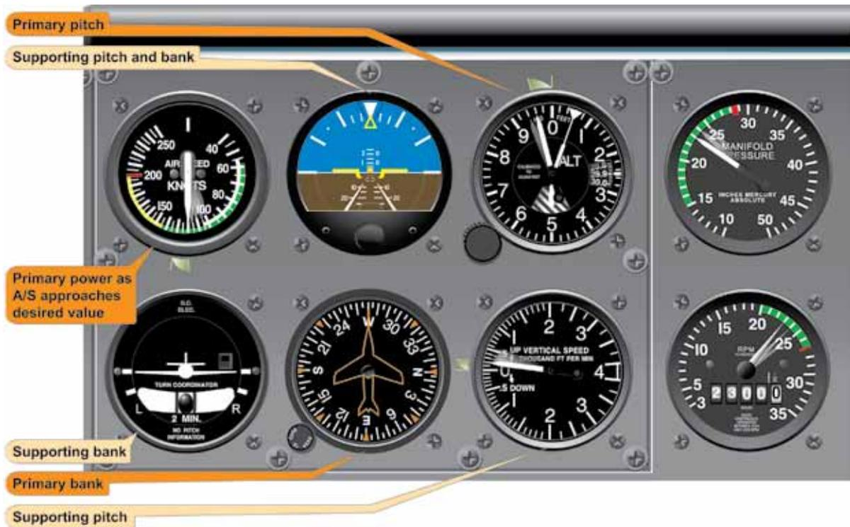
**Figure 5-29.** Level Off at Cruising Speed.
