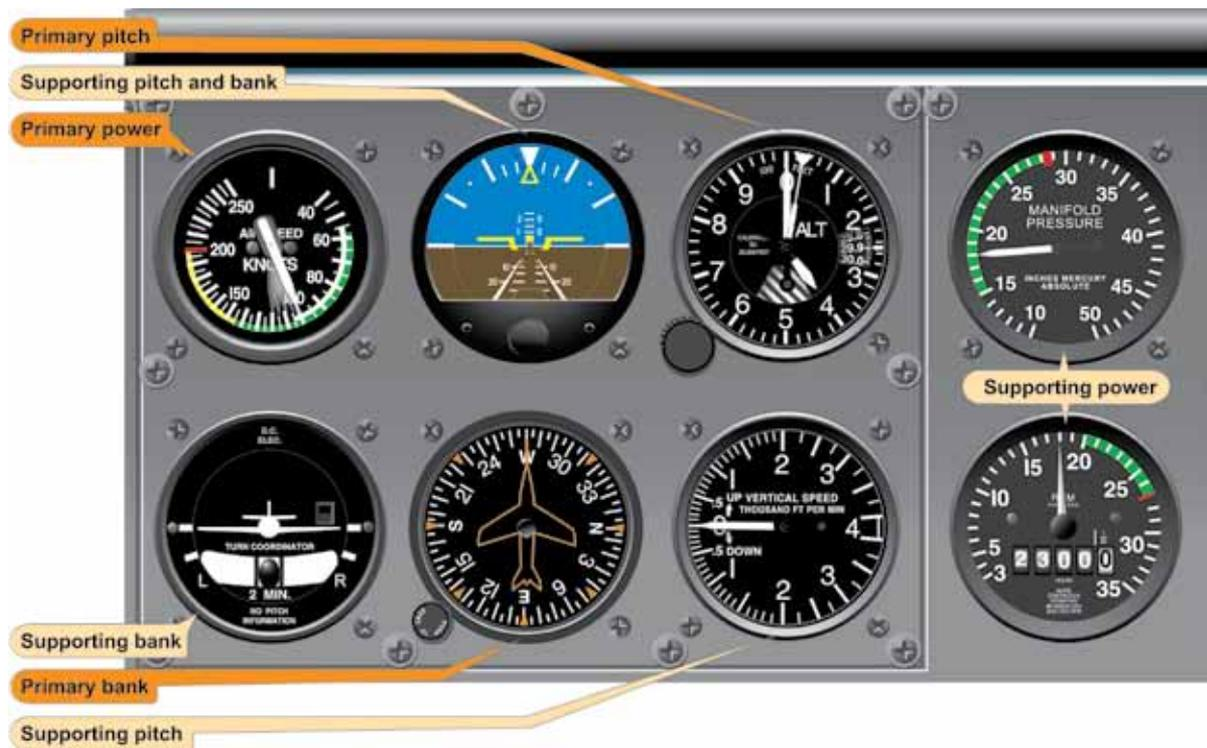
**Figure 5-24.** *Straight-and-Level Flight (Reduced Airspeed Stabilized).*
