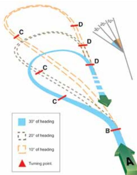
**Figure 5-44.** Teardrop Pattern (Entire Pattern in Level Flight).
