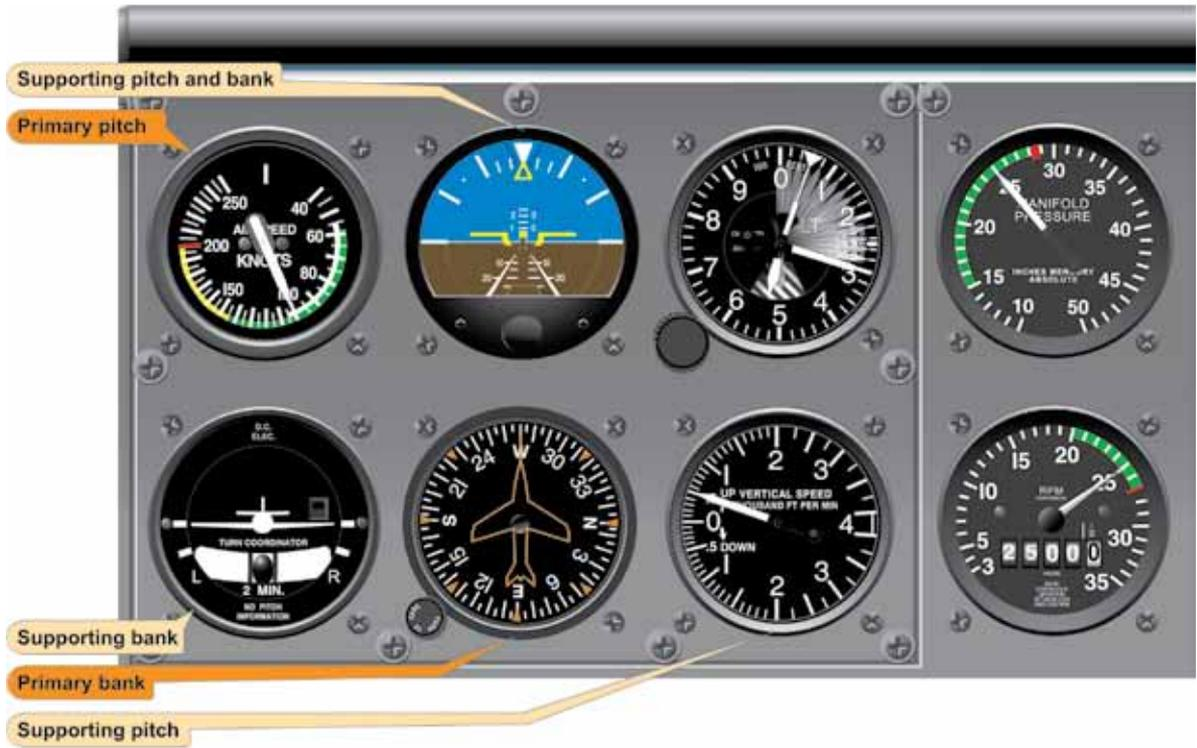
Figure 5-26. *Stabilized Climb at Constant Airspeed.*
