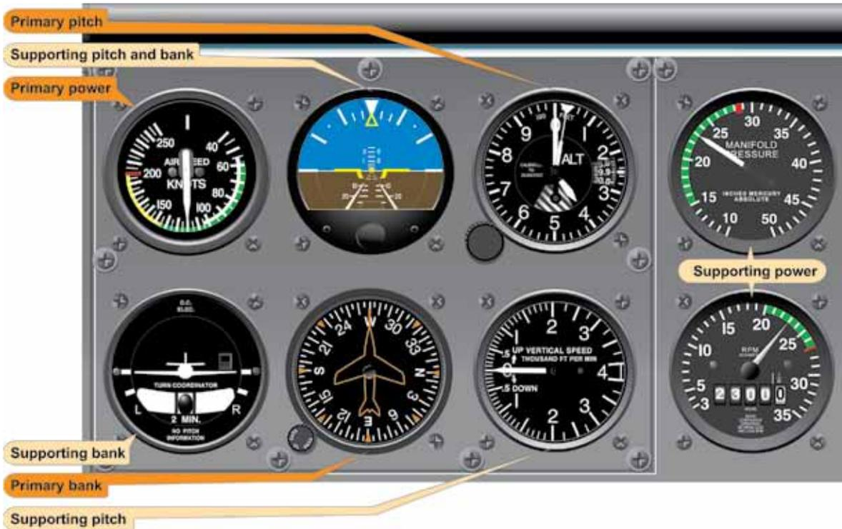
Figure 5-22. Straight-and-Level Flight (Normal Cruising Speed).
