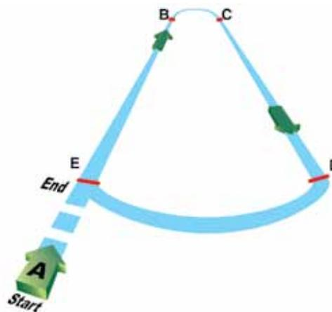
Figure 5-41. Racetrack Pattern (Entire Pattern in Level Flight).
