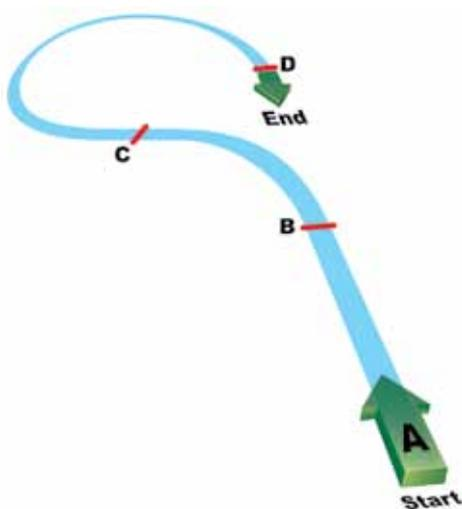
**Figure 5-43.** 80/260 Procedure Turn (Entire Pattern in Level Flight).
