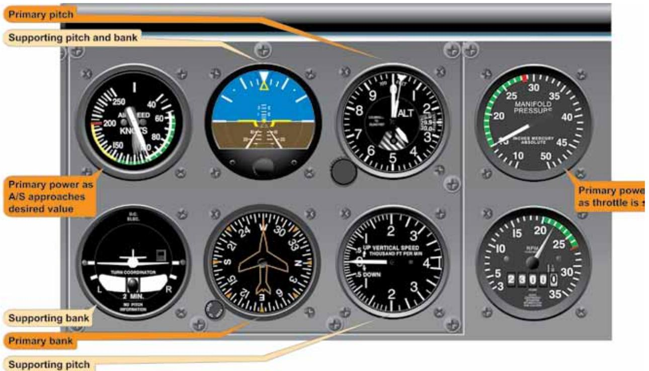
Figure 5-23. Straight-and-Level Flight (Airspeed Decreasing).
