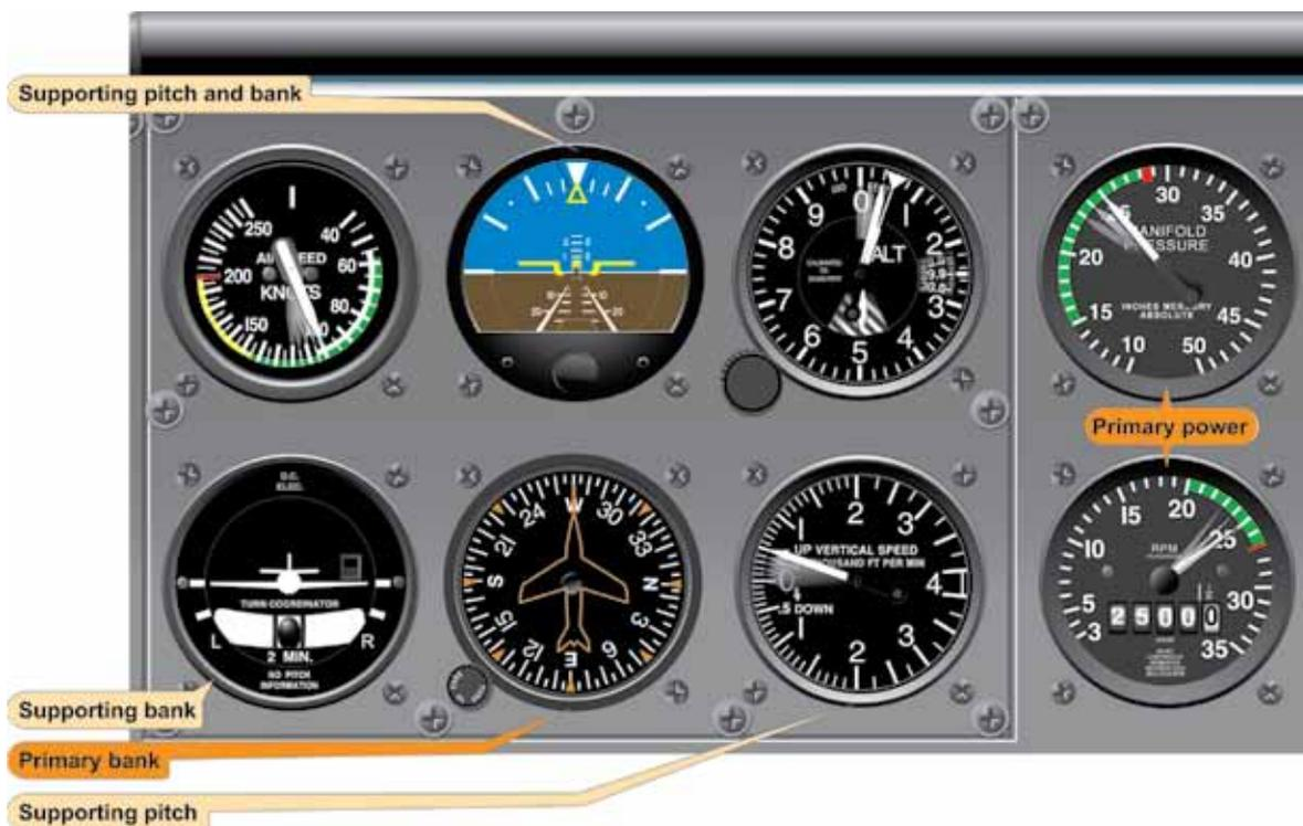
Figure 5-25. Climb Entry for Constant Airspeed Climb.
