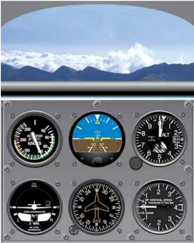
Figure 5-1. Pitch Attitude and Airspeed in Level Flight, Slow Cruise Speed.
