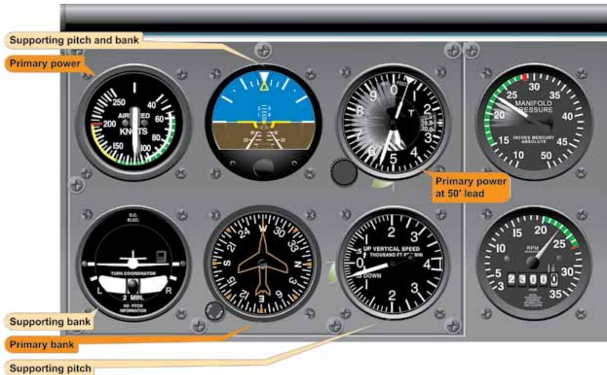
Figure 5-32. Level Off at Descent Airspeed.
