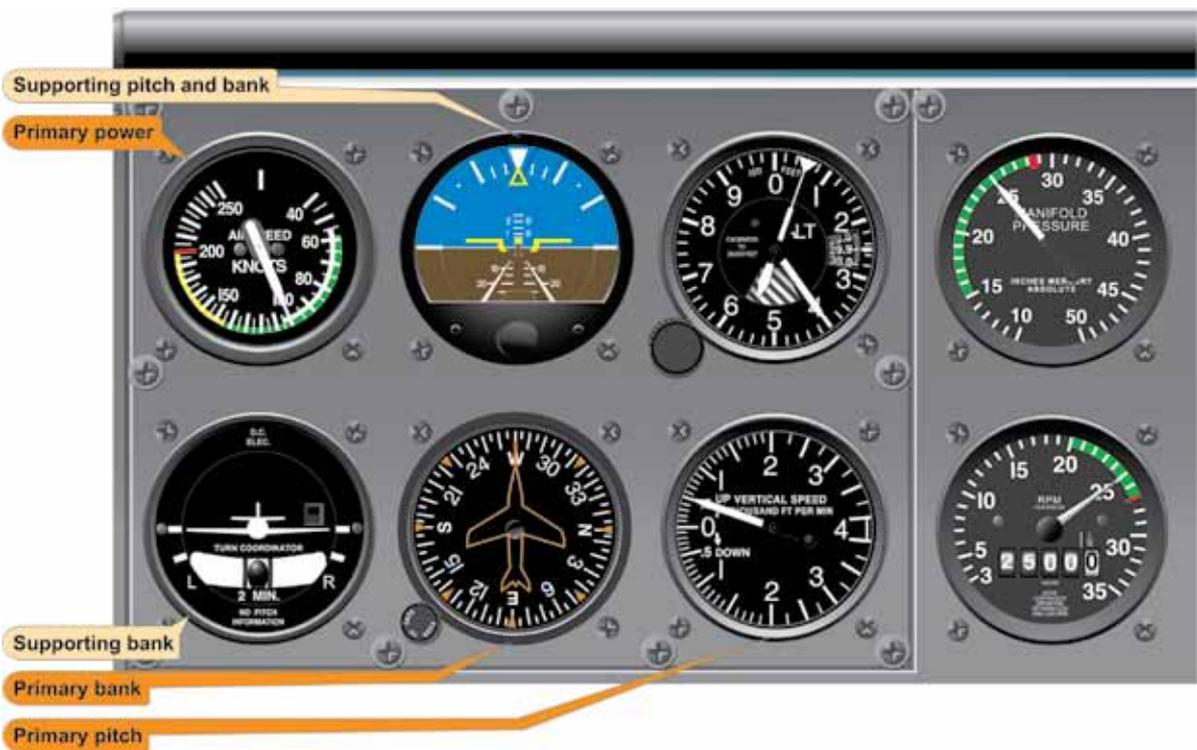
Figure 5-27. *Stabilized Climb at Constant Rate.*
