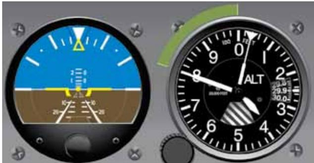
**Figure 5-11.** *Altitude Error, Greater Than 100 Feet.*
