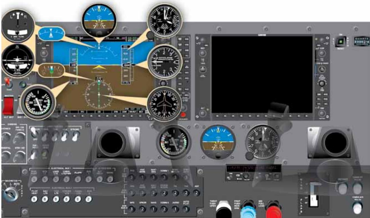
Figure 4-21. Primary Flight Display (PFD) and Analog Counterparts.
