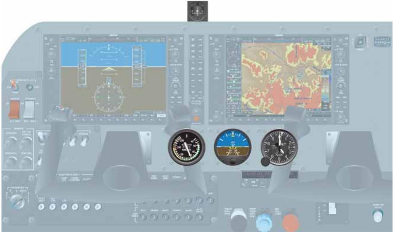
**Figure 4-24.** Emergency Back-up of the Airspeed Indicator, Attitude Indicator, and Altitude Indicator.
