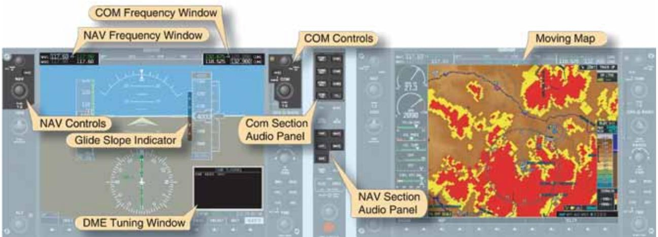
**Figure 4-27.** Navigation Instruments.
