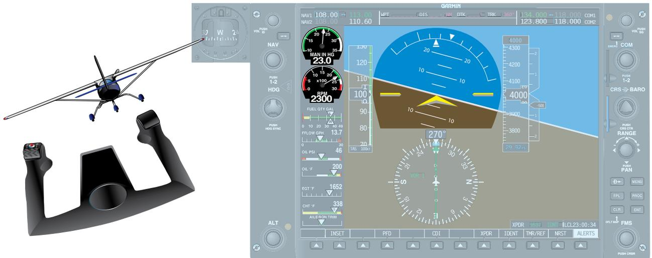
**Figure 4-25.** Control Instruments.
