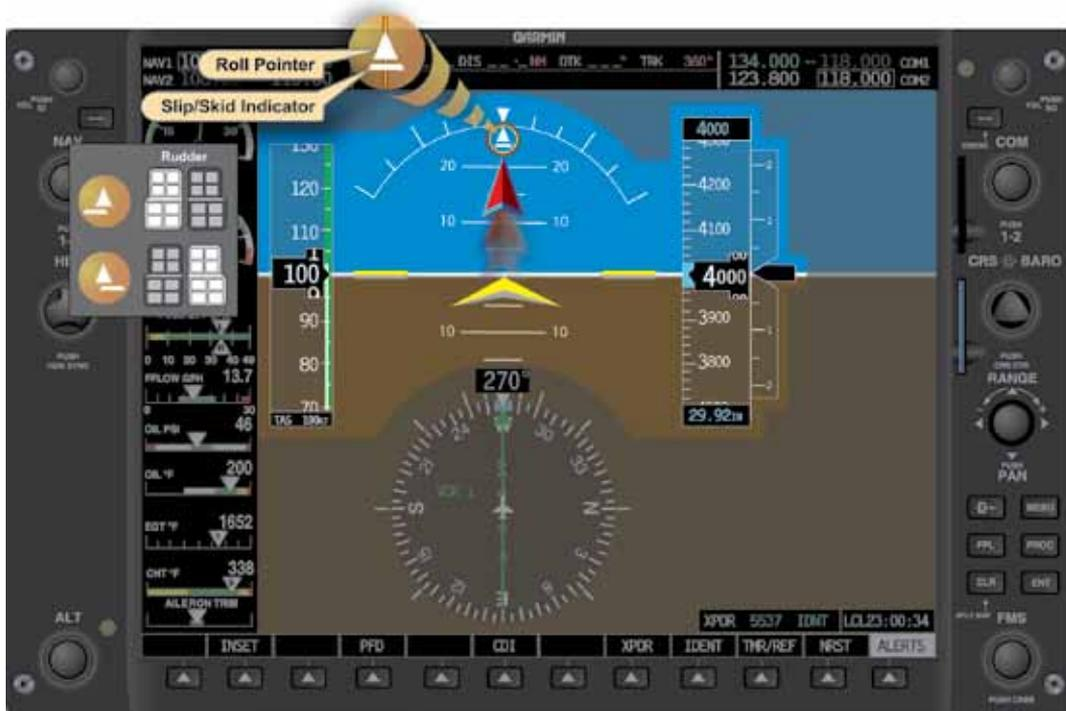
Figure 4-35. Roll Pointer and Slip/Skid Indicator.
