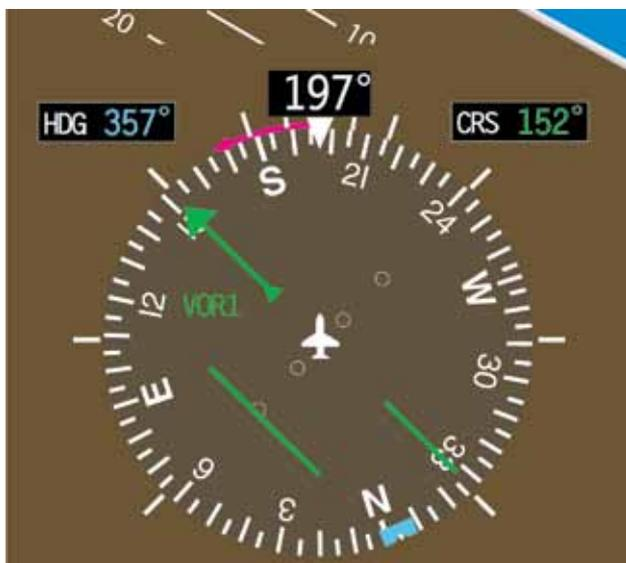
Figure 4-40. HSI Indicator (enlargement).
