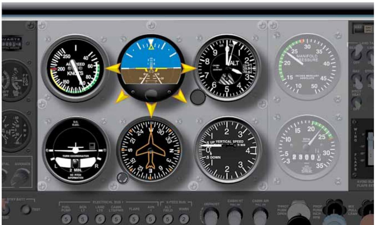
Figure 4-17. Radial Cross-Check.
