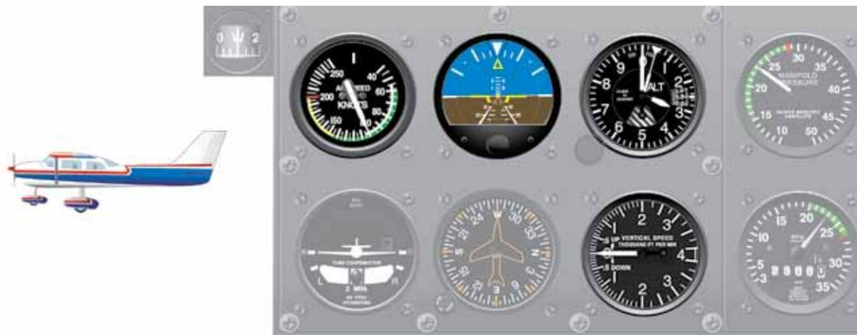
**Figure 4-4.** Pitch Instruments.
