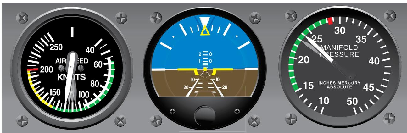
Figure 4-13. An Increase in Power Increasing Airspeed Accordingly in Level Flight.
