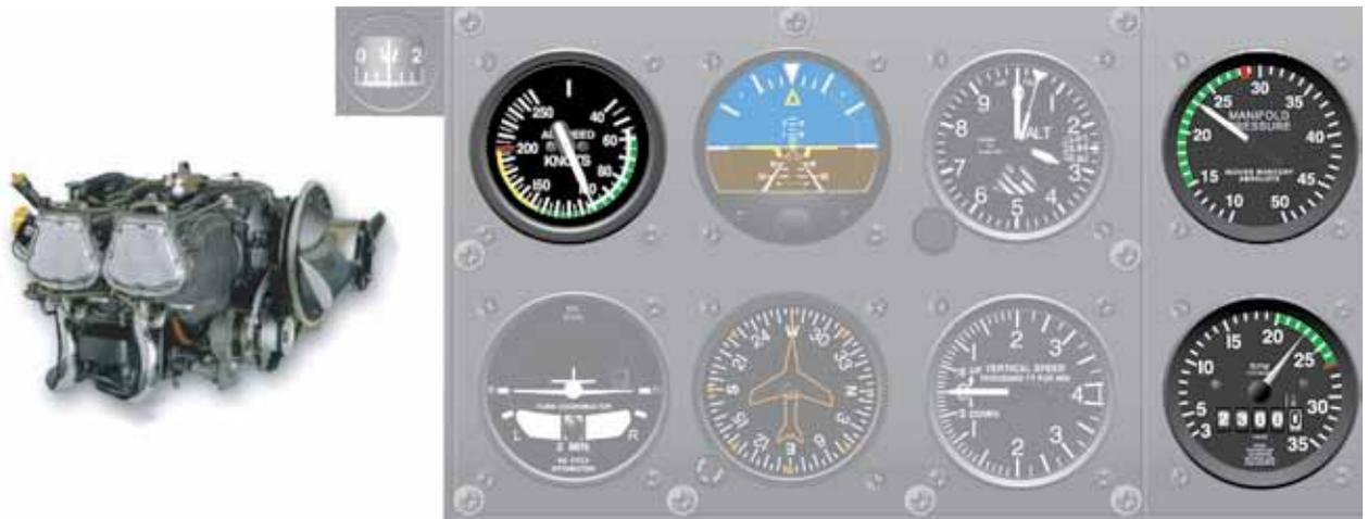
Figure 4-15. Power Instruments.
