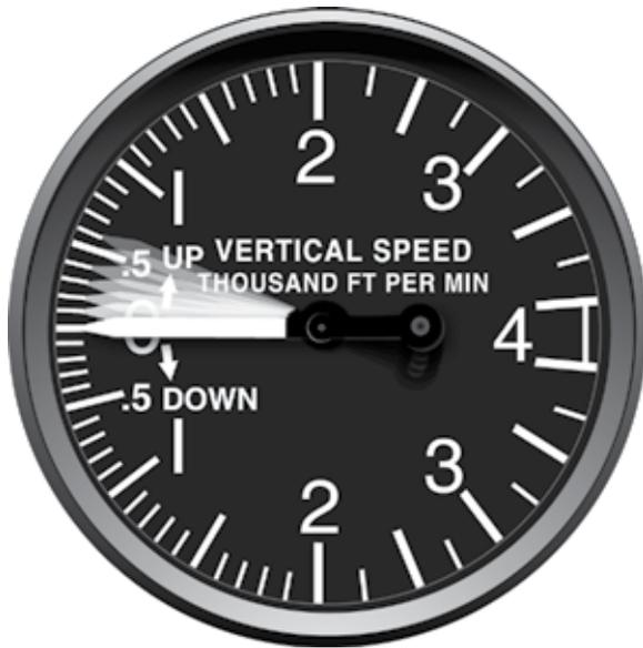
**Figure 4-8.** Vertical Speed Indicator.
