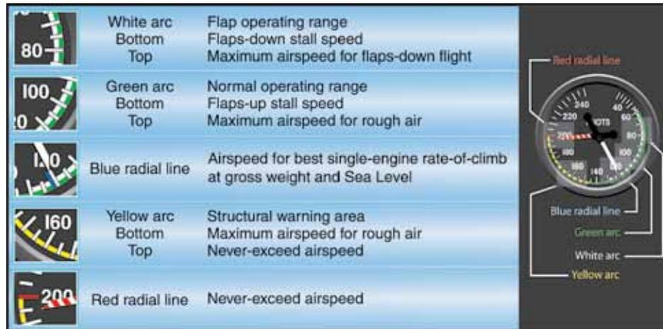
**Figure 3-15.** *Color Codes for an Airspeed Indicator.*
