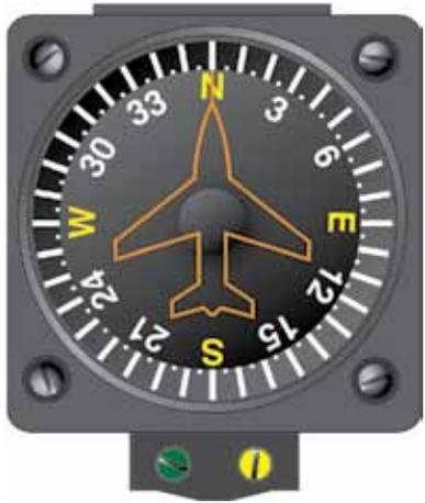
**Figure 3-22.** Vertical Card Magnetic Compass.
