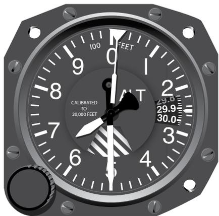
**Figure 3-4. Three-Pointer Altimeter.**
