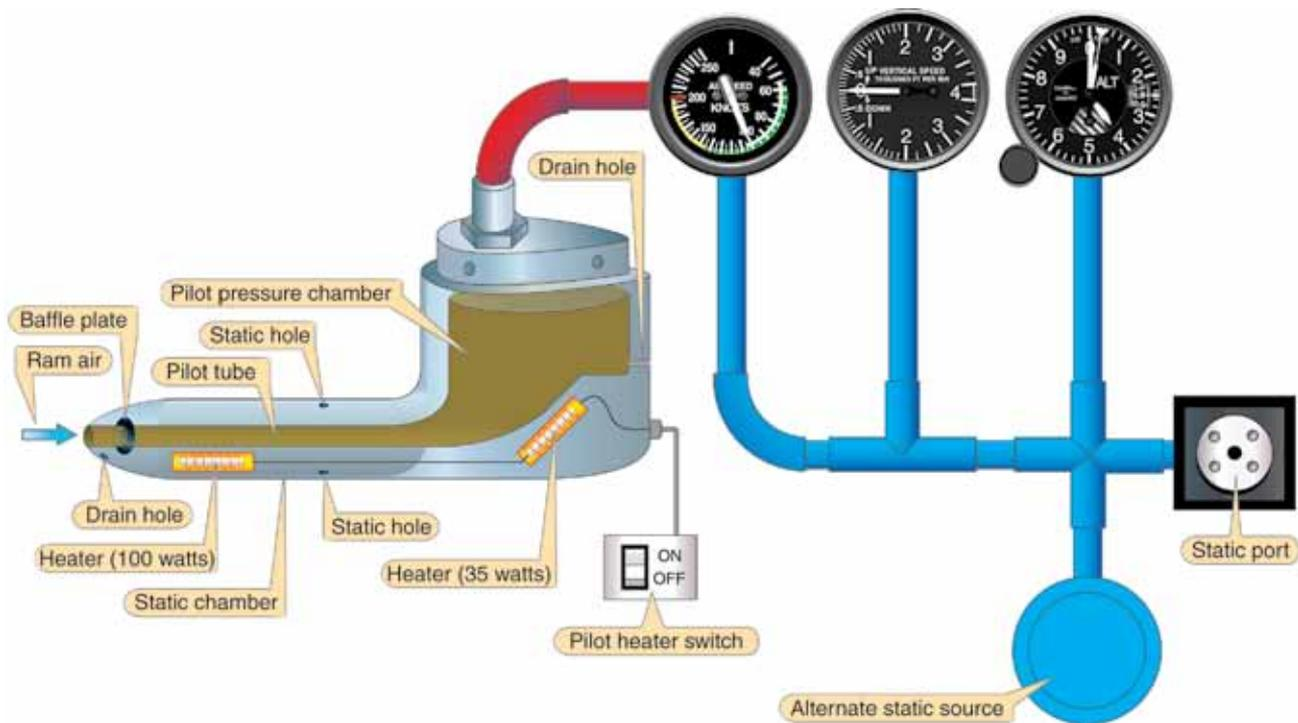
Figure 3-1. A Typical Electrically Heated Pitot-Static Head.
