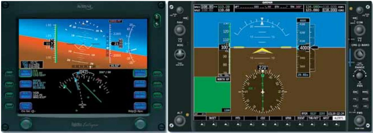
Figure 3-45. Two Primary Flight Displays (Avidyne on the Left and Garmin on the Right).
