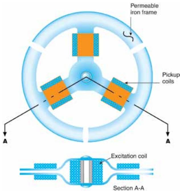
**Figure 3-23.** The soft iron frame of the flux valve accepts the flux from the Earth's magnetic field each time the current in the center coil reverses. This flux causes current to flow in the three pickup coils.
