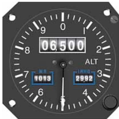
**Figure 3-5. Drum-Type Altimeter.**
