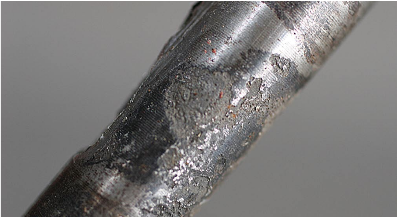
Figure 6-7. Dissimilar metal corrosion.
