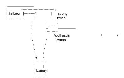
When the flat piece of wood is removed by pulling the string, the jaws of the clothespin will close, completing the circuit.
