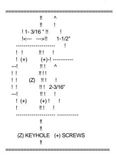
AFTER THIS IS ACCOMPLISHED, THE LOCK CAN BE PUSHED BACKWARDS DISENGAGING THE LOCK FROM THE COVER PLATE. THE FOUR BOLTS OF THE COVER PLATE CAN THEN BE RETRACTED BY TURNING THE BOLTWORKS WITH A SIMPLE KEY IN THE SHAPE OF THE HOLE ON THE COIN PLATE (SEE DIAGRAM BELOW). OF COURSE, THERE ARE OTHER METHODS AND DRILLING PATTERNS.
