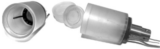
Fig. 6.15. A plastic mixing chamber for a dilution unit.
