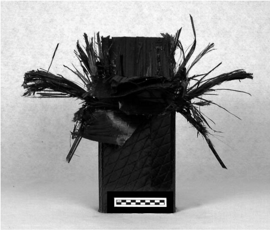
Fig. 6.8. Carbon fiber reinforced box beam after longitudinal crushing in a drop tower experiment.
