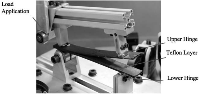
Fig. 6.13. Set-up of a double cantilever beam test. (Reprint with permission from Peter [305])
