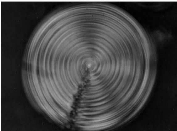
Figure 13.21. Cholesteric monopole in a droplet (Robinson spherulite) with a disclination k = 2 in the director field. Droplet radius about 30\mu\text{m} .
