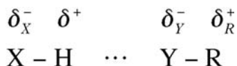
Figure 1.11. A hydrogen bond between two atomic groups XH and YR that contain strongly electronegative atoms (X and Y).
