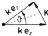
Figure 9.12: Angle-relations for the calculation of the scattering amplitude in the first Born approximation
