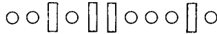
FIG. 5.07. Schematic model for calculating the number of ways of distributing n energy units among \Delta N modes. In this illustration, n = 7 and \Delta N = 5 . The seven open circles symbolize energy units and the four vertical bars are separators which divide the set of circles into five disjoint subsets. Here the populations of the subsets are (from left to right) 2, 1, 0, 3, and 1, respectively.
