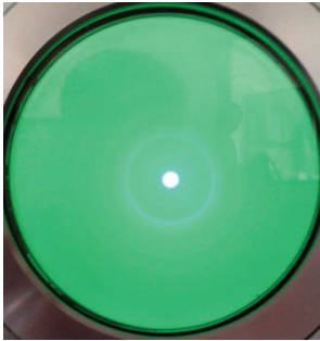
Figure 2.4. Electron diffraction pattern (unaffected by magnetic field).
