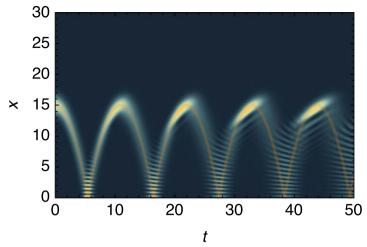
The orange overlaid curve shows the classical particle trajectory from In [490], which the quantum particle follows approximately while self-interfering during the reflections.
