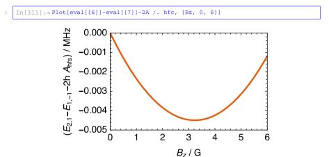
At the "magic" field strength  $B_0 = 3.228\,96\,\mathrm{G}$  the energy difference is independent of the magnetic field (to first order):
