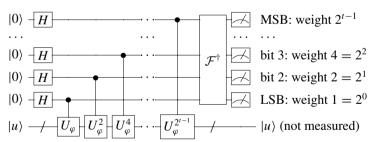
To set up a quantum phase estimation in Mathematica, we begin by defining the unitary operator  $\hat{U}_{\varphi}$  and its eigenstate  $|u\rangle$  with
