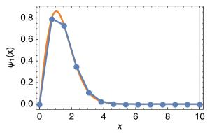
You can see that even with  $n_{\text{max}} = 12$  grid points this ground-state wavefunction (blue lines interpolating between blue calculated points) looks remarkably close to the exact one (orange line, see plot on page 103).
