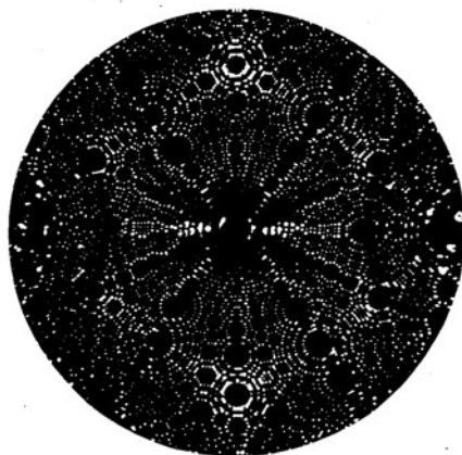
Figure 11.13. Field ion microscope image of a tungsten tip of radius \sim 400 \text{ \AA} . The original image had a magnification of 3 million. (Photo courtesy of T. Tsonq.)
