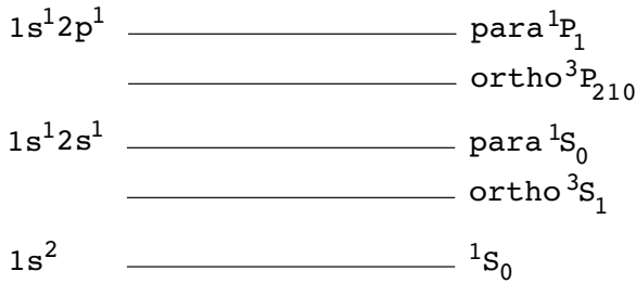
FIGURE 18.1 Energy levels for low-lying configuration of the helium atom.
