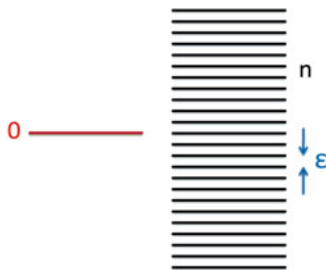
Fig. 24.1 Discrete state 0 coupled to a discrete continuum of states labeled by n . The energy difference between successive levels is \epsilon
