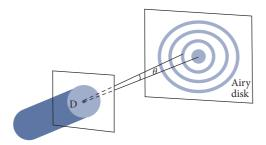
Fig. 4.16 Diffraction from a circular aperture.
