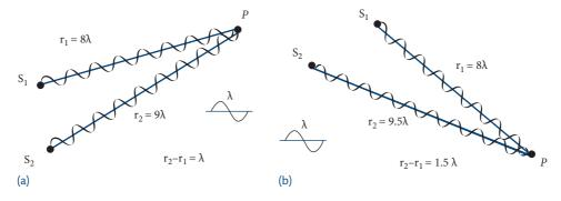
**Fig. 4.6** Two waves of wavelength  $\lambda$  originate from points  $S_1$  and  $S_2$ . (a) If, at point P the difference in the distance travelled from  $S_1$  and  $S_2$  is equal to  $\lambda$ , there is constructive interference and (b) if the distance is equal to 1.5  $\lambda$ , there is destructive interference.
