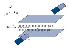
Fig. 3.11 An electron passing through a region of magnetic field is deflected in a direction perpendicular to both its velocity and the magnetic field.
