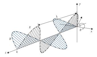
**Fig. 9.2** Polarization is along the direction **E** making an angle  $\theta$  with the x-axis.
