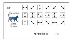
**Fig. 13.6** A quantum currency note has a serial number and a number of trapped photons each stored in one of the four BB-84 states  $|\rightarrow\rangle$ ,  $|\nearrow\rangle$ ,  $|\uparrow\rangle$ ,  $|\uparrow\rangle$ .
