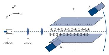
**Fig. 3.12** A collimated electron beam passes through a region where both electric and magnetic fields are applied. The fields are set up in such a way that the electric field and the magnetic field forces on the electron are adjusted such that the net force on the electron in the y-direction is zero.
