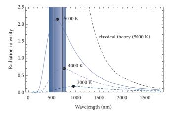
**Fig. 6.4** The spectral distribution  $J(\nu, T)$  as a function of wavelength. The emitted radiation peaks at shorter wavelength (higher frequency) with increasing temperature. According to classical theory the emitted radiation approaches infinity as the wavelength decreases leading to "ultraviolet catastrophe".
