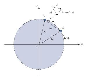
**Fig. 3.7** In a uniform circular motion of a particle, the velocity changes from  $\mathbf{v}_i$  to  $\mathbf{v}_f$ . The change in velocity  $\Delta \mathbf{v} = \mathbf{v}_f - \mathbf{v}_i$  points towards the center of the circular path.
