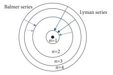
**Fig. 6.12** According to the Bohr model of atom, the electrons exists only in prescribed orbits of radii  $r_n$ . Each orbit has a definite energy. When an electron jumps from a higher level to a lower level, a photon of energy equal to the energy difference between the two levels is emitted.
