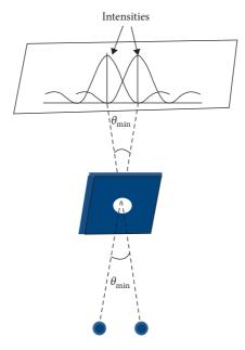
**Fig. 4.19** Images formed by two point sources through a circular aperture are Airy patterns. According to the Rayleigh criterion, the two point sources can be resolved if the principal diffraction maximum of one image coincides with the first diffraction minimum of the second image.
