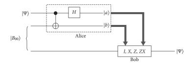
**Fig. 15.7** Circuit diagram for the quantum teleportation of the state  $|\psi\rangle$  from Alice to Bob. A Bell basis state  $|B_{00}\rangle$  is created between Alice and Bob. Alice makes a joint Bell basis measurement on the two qubits at her end and conveys the outcome to Bob via a classical channel. Bob transforms his state by applying I, X, Z, and ZX gates depending on Alice's measurement and recovers the state  $|\psi\rangle$ .
