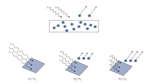
**Fig. 6.5** Photoelectric effect: When light is incident on a metal, photoelectrons are emitted. No electrons are emitted if the frequency of light is below a critical frequency. At the critical frequency, the electron emission starts. As the frequency of light is increased further, the kinetic energy of the emitted electrons is also increased.
