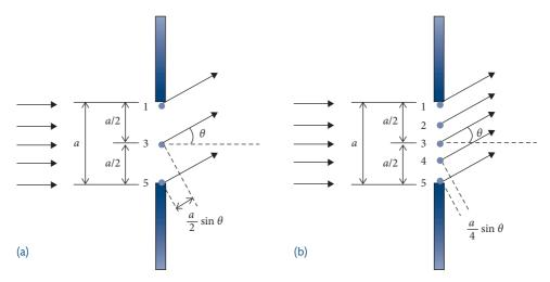
**Fig. 4.13** Condition for a dark spot in the diffraction of light from a single slit. (a) The condition for destructive interference is satisfied for light originating from points 1 and 3 as well as 3 and 5 and (b) the condition for destructive interference is satisfied for light originating from points 1 and 2, 2 and 3, 3 and 4, and 4 and 5.
