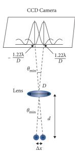
**Fig. 7.10** The uncertainty of the position of the electron is determined by using the Rayleigh criterion. The minimum uncertainty  $\Delta x$  subtends an angle  $\theta_{min}$  with the lens.
