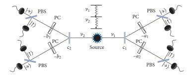
Fig. 12.7 Schematics for an experiment to test the CHSH inequality.
