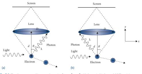
**Fig. 7.9** The photon scattered in any angle ranging from  $+\theta$  to  $-\theta$  with the vertical is detected. (a) The minimum momentum is imparted to the electron by those photons that are scattered at the angle  $+\theta$  whereas (b) maximum momentum is imparted by photons scattered at the angle  $-\theta$ .
