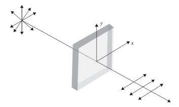
Fig. 9.3 Unpolarized light passing through a polarizer with its polarizing axis along the x-axis.
