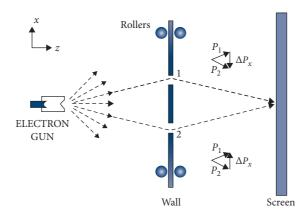
**Fig. 8.6** Einstein's *gedanken* experiment. Electrons pass through a narrow slit through a wall that can freely move on a roller. The momentum transfer to the wall provides the which-path information. At the same time electrons from the two slits can form an interference pattern on the screen.
