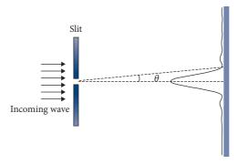
Fig. 4.12 Diffraction of light from a single slit.
