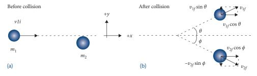
**Fig. 7.12** A particle of mass  $m_1$  moving with a velocity  $v_{1ix}$  collides with another particle of mass  $m_2$  at rest. The scattered particles move in directions making angles  $\theta$  and  $\phi$  with the horizontal.
