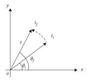
**Fig. 3.4** A particle undergoes an angular displacement from  $\theta = \theta_i$  at time  $t_i$  to  $\theta = \theta_f$  at a later time  $t_f$ .
