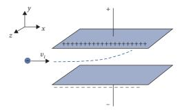
Fig. 3.9 An electron passing through a region of electric field is deflected towards the positively charged plate.
