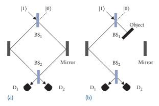
**Fig. 14.2** (a) In a Mach–Zehnder interferometer, a photon incident on a beam splitter  $BS_1$  is reflected by mirrors, recombined at the second beam splitter  $BS_2$ , and is detected either at detector  $D_1$  or  $D_2$ . (b) The same set-up as in (a) but with a photon absorber on the right-hand side of the interferometer.
