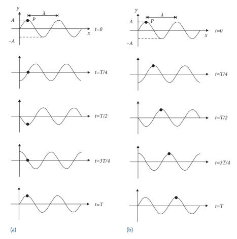
**Fig. 4.3** A transverse wave of amplitude A and wavelength  $\lambda$  is depicted at different times. (a) A point on a wave undergoes a full oscillation during the time period T. (b) T is also the time period in which the wave propagates through a distance  $\lambda$ .
