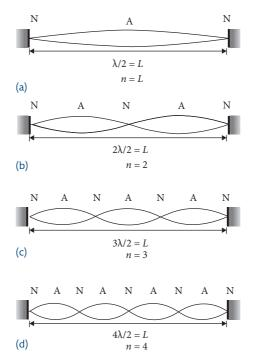
Fig. 4.8 Standing waves with (a) one antinode, (b) two antinodes, (c) three antinodes, and (d) four antinodes.
