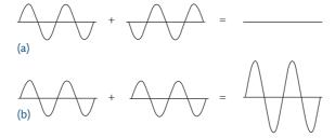
**Fig. 4.5** Superposition of two waves. (a) The two waves are displaced by a distance equal to half the wavelength,  $\lambda/2$ , and the two waves cancel each other at every point, resulting in a wave of zero magnitude. (b) The two waves are displaced by a distance equal to the wavelength,  $\lambda$ , and the two waves superimpose on each other yielding a wave of twice the amplitude.
