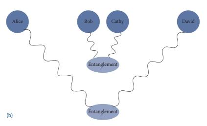
**Fig. 10.6** Entanglement swapping: (a) Entangled states are prepared between Alice and Bob's photons as well as between Cathy and David's photons. A Bell state measurement is made between Bob and Cathy. (b) The result is that, after the measurement is made, the previous entanglements disappear and new entangled states are formed between Alice and David and between Bob and Cathy.
