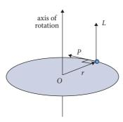
Fig. 3.8 Angular momentum  $\boldsymbol{L}$  is perpendicular to the plane containing the linear momentum  $\boldsymbol{p}$  and the position vector  $\boldsymbol{r}$ .
