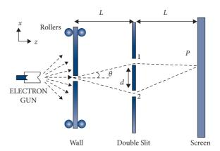
**Fig. 8.7** An analysis of Einstein's *gedanken* experiment. Electrons pass through a wall giving it a push in the upward or the downward direction depending on whether the incoming electron is scattered in the downward or upward direction. This provides the which-path information. These electrons then pass the double slit and form a pattern on the screen.
