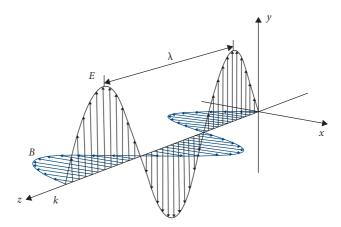
**Fig. 9.1** An electromagnetic wave. Electric and magnetic fields, **E** and **B**, oscillate in directions mutually perpendicular to each other as well as perpendicular to the direction of propagation of the wave vector **k**.
