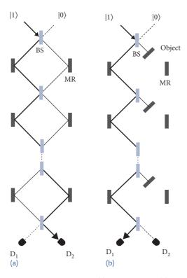
**Fig. 14.3** (a) An array of N Mach–Zehnder interferometers. (b) Same set-up as in (a) but with an absorber at each step such that if the photon leaks to the right-hand side, it is absorbed.
