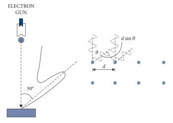
**Fig. 7.3** The result of the Davisson–Germer experiment can be explained by treating electrons as de Broglie waves of wavelength  $\lambda_{dB} = h/mv$  that are diffracted by the atoms inside the crystal and are scattered at those angles  $\theta_n$  where the condition of constructive interference is satisfied.
