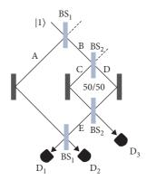
A single photon is incident as shown in the figure. Both the beam splitters  $BS_2$  are 50/50 beam splitters whereas the beam splitters  $BS_1$  have transmission and reflections amplitudes t and r.
