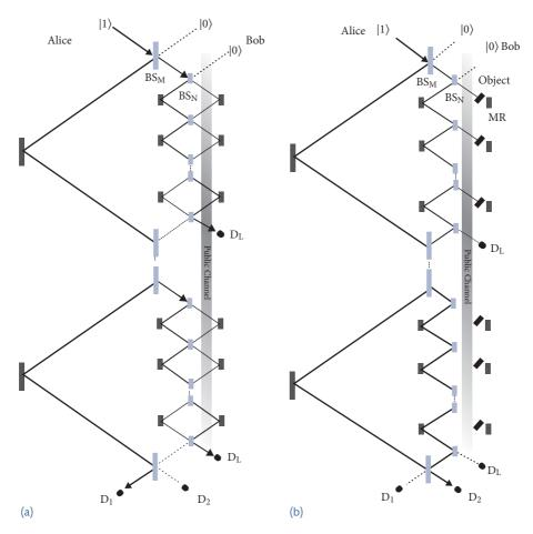
**Fig. 14.4** A double array of Mach–Zehnder interferometers for counterfactual communication. Here Alice sends the photon and Bob decides whether to send (a) bit "1" by not blocking the mirrors and (b) bit "0" by absorbing the photon if it enters the Bob side of the interferometer.
