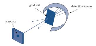
**Fig. 6.8** Schematics of Rutherford's experiment. A beam of alpha particles is incident on a thin sheet of gold. An array of detectors detect alpha particles after they scatter from the gold foil.
