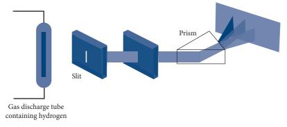
**Fig. 6.10** Schematics for observing the emission spectrum of hydrogen. A gas discharge tube containing hydrogen emits radiation which is first collimated by narrow slits and then passed through a prism which deflects light of different frequencies in different directions.
