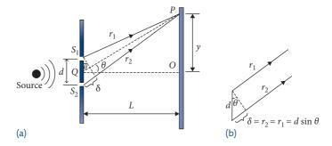
**Fig. 4.10** The path difference from light originating from slits  $S_1$  and  $S_2$  is equal to  $d \sin \theta$  in the limit when  $L \gg d$ .
