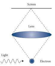
**Fig. 7.8** Heisenberg microscope. The position of the electron is determined from the light that is scattered from an electron into the lens.
