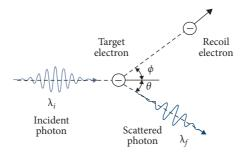
**Fig. 7.11** Compton scattering: A photon of wavelength  $\lambda_i$  is scattered by an electron at rest making an angle  $\theta$  with the horizontal and with a final wavelength  $\lambda_f$ .
