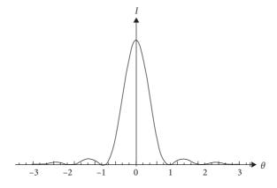
Fig. 4.15 The diffraction pattern as given by Eq. (4.63).
