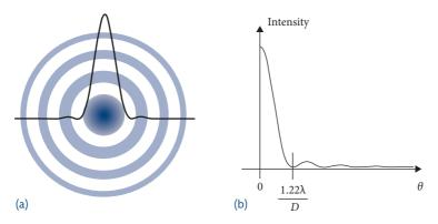
**Fig. 4.17** The diffraction pattern from a circular aperture is the Airy pattern (4.67). (a) There is a bright spot at the center followed by alternating dark and bright spots. (b) The first dark spot is located at  $\theta = 1.22 \lambda/D$ .
