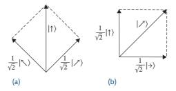
**Fig. 10.3** (a) A photon in state  $|\uparrow\rangle$  can be looked upon as a superposition of  $|\nearrow\rangle$  and  $|\nwarrow\rangle$  states; (b) A photon in state  $|\nearrow\rangle$  can be looked upon as a superposition of  $|\rightarrow\rangle$  and  $|\uparrow\rangle$  states.
