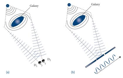
**Fig. 8.8** Wheeler's delayed choice experiment. Light that left a quasar millions of years ago can be made to act like a particle or a wave depending on our choice of the experimental set-up.
