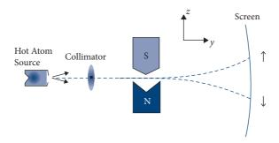
**Fig. 5.1** Schematics of Stern–Gerlach experiment. An electron is deflected by an inhomogeneous magnetic field in the "up" direction or in the "down" direction depending on whether it is in the state  $\psi_1$  or in the state  $\psi_1$
