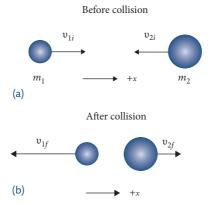
Fig. 3.2 Collision between two particles in one dimension.
