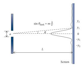
Fig. 4.14 In the diffraction pattern from a slit of width a, the dark spots are equidistant.
