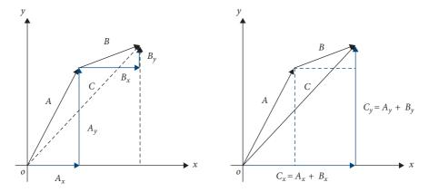
Fig. 2.10 Sum of two vectors A and B via component method.
