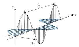
**Fig. 6.3** Light is an electromagnetic wave with the mutually perpendicular electric and magnetic fields oscillating in the directions normal to the direction of propagation.
