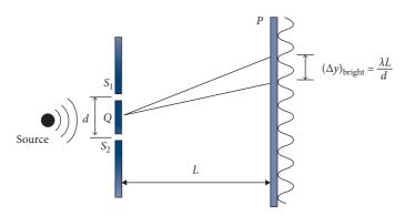
**Fig. 4.11** The spacing between the maxima of the adjacent fringes in Young's double-slit experiment is equal and given by  $\lambda L/d$ .
