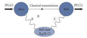
**Fig. 10.5** Teleportation of a state  $|\psi(A)\rangle$  at Alice's end to Bob's end. An entangled state  $|B_{00}(B,C)\rangle$  is generated, particle B goes to Alice and particle C goes to Bob. Alice announces the outcome of the Bell basis measurement for states A and B to Bob on a classical channel. Bob makes local adjustments on his particle C accordingly and the state  $|\psi(A)\rangle$  is teleported to Bob.
