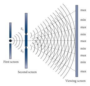
**Fig 4.9** In Young's double-slit experiment, light from a source is incident on a screen with two slits. The light from these slits forms an interference pattern on the viewing screen.
