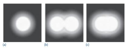
**Fig. 4.18** (a) Diffraction pattern from a single point. (b) Diffraction pattern from two points whose separation is large enough that they can be resolved, and (c) when they cannot be resolved.
