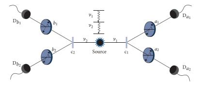
Fig. 12.6 Schematics for an experiment to test Bell's inequality.
