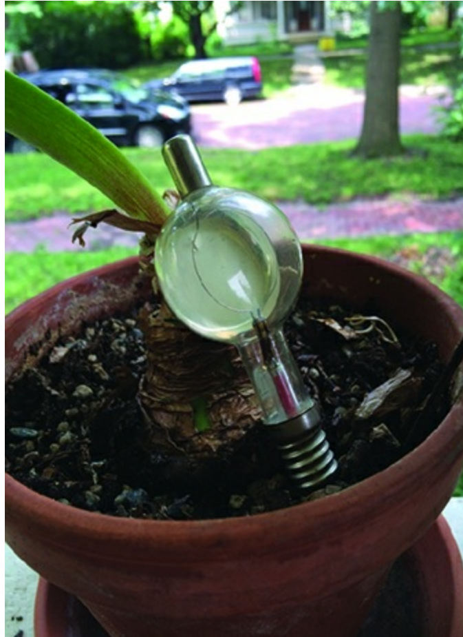
Figure 2.5. A quaint 1930s phototube in a flower pot. Light shining on the metal backing kicks electrons out to the wire loop, which has a voltage set up to attract them. An atom explodes because of a resonance between its time dependence and the light.
