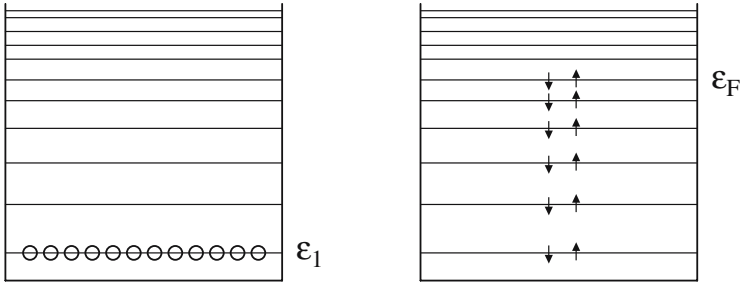
Fig. 16.3. Ground state of a system of N independent identical particles. Left: bosonic case, with all the particles in the ground state of the one-body Hamiltonian. Right: fermionic case, where the first N/(2s+1) states of the one-body Hamiltonian are occupied (here s = 1/2 )
