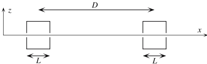
Fig. 17.4. Experimental setup for the observation of Ramsey fringes
