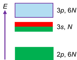
Fig. 9.14 Bands formed by the combination of orbitals on sodium atoms. A green color signifies that a band or portion of the band is filled, whereas a red color signifies a portion of the band that is empty. The band arising from the 3s orbitals is only half filled, because there is only one electron in the 3s state of each sodium atom. The band from combination of 3p states is empty. (Modified with permission from House, J. E. Inorganic Chemistry , 2nd ed.; Academic Press/Elsevier: Amsterdam, 2013.)
