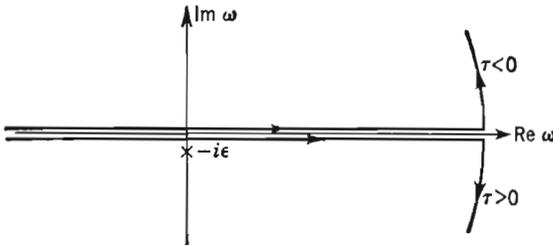
Fig. 6-2 Contour in the complex  $\omega$  plane for integrating the unit step function  $\theta(\tau)$ .
