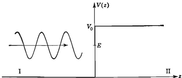
Fig. 3-2 Electrostatic potential idealized with a sharp boundary, with an incident free electron wave of energy  $E$  moving to the right in region I. For  $V_0 > E + mc^2$  the reflected current from the potential exceeds the incident one; this is an example of the Klein paradox.
