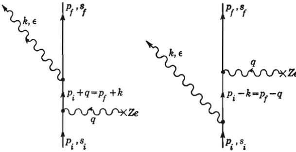
Fig. 7-8 Bremsstrahlung of an electron in a Coulomb field.
