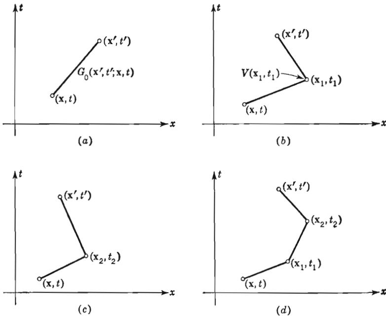
Fig. 6-1 Space-time diagrams for propagation from  $(\mathbf{x}, t)$  to  $(\mathbf{x}', t')$  as (a) a free particle, (b) with one scattering by potential  $V(\mathbf{x}_1, t_1)$  at  $(\mathbf{x}_1, t_1)$ , (c) with single scattering at  $(\mathbf{x}_2, t_2)$ , and (d) with double scattering.
