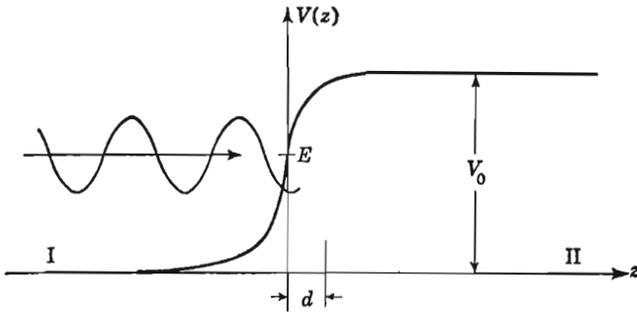
Fig. 3-1 Potential barrier confining electron of energy  $E$  in region I to the left.
