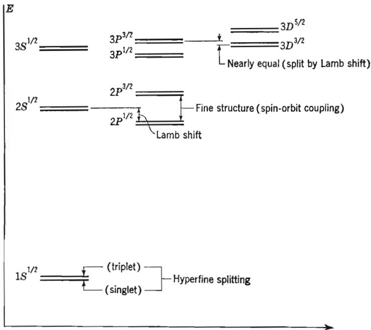
Fig. 4-2 Low-lying energy levels of atomic hydrogen. The diagram is not drawn to scale.
