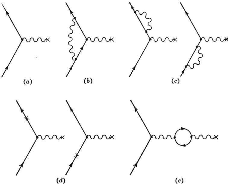
Fig. 8-10 Second-order radiative corrections to scattering in an external electromagnetic potential.
