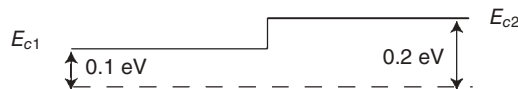
FIGURE 1.8 A junction formed by two n-type semiconductors with different doping levels. The material on the left has heavier doping because the Fermi level (dashed line) is closer to the conduction band.
