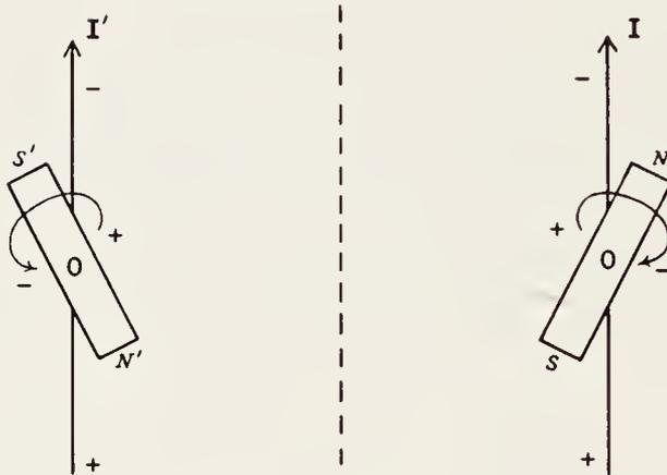
FIG. 14.2. Deflection of a magnetic dipole by a current and mirror image of this process (assuming charge to be a scalar).
