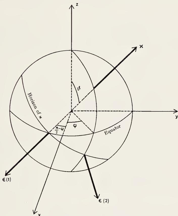
FIG. 18.1. The polarization vectors  $\epsilon(1)$  and  $\epsilon(2)$  characterizing transverse fields propagating in direction  $\mathbf{x}$ .
