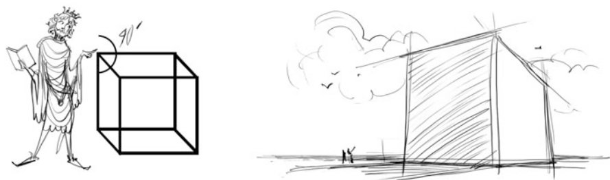
Fig. 1.2 Orthogonal versus perspective views
