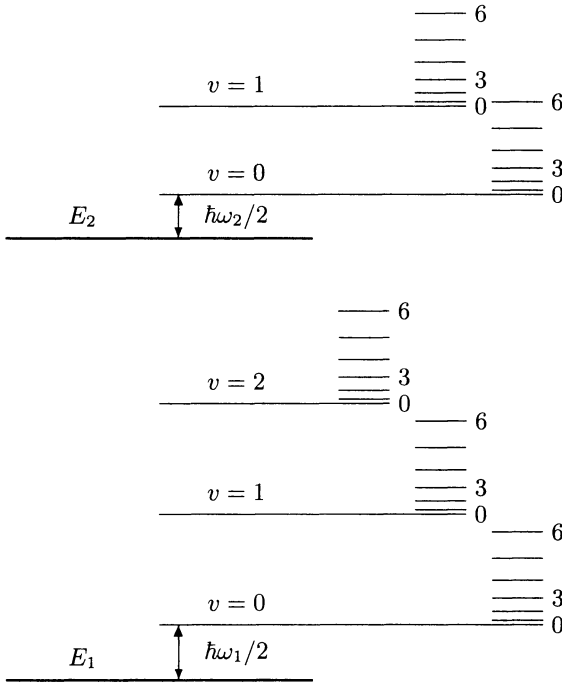
Fig. 20.4. Energy levels of a diatomic molecule. Numbers on the right are values of J
