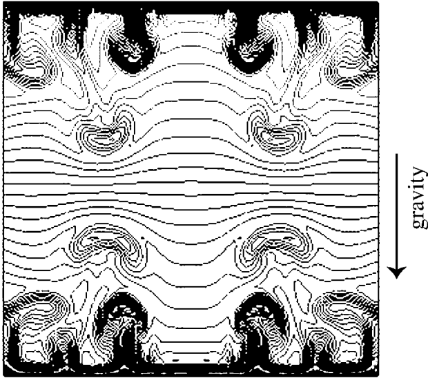
Fig. 6.16. Thermal plumes in CO 2 in a cell with 1 cm thickness in an initial stage of the Schwarzschild instability. The darkness in the figure may be interpreted to represent |T(\mathbf{r}, t) - T_{\text{center}}(t)| where T_{\text{center}}(t) is the temperature at the center. (The original figure in [67] is in color and represents T(\mathbf{r}, t) - T_0 .) The temperature inhomogeneity is of order 0.5 mK and is much smaller than the average deviation T - T_c = 1 K.
