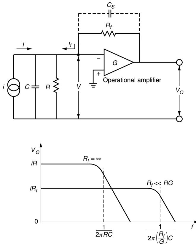
Figure 16.16 Transimpedance coupling.
