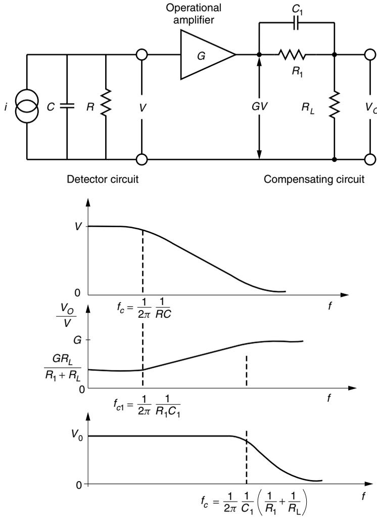
Figure 16.15 High impedance with a compensation circuit.
