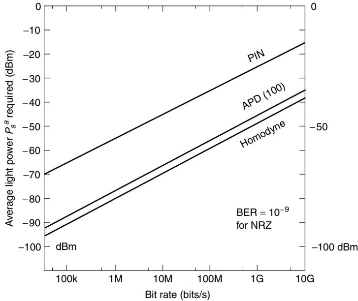
**Figure 16.30** Input average light power  $P_s^a$  versus bit rate (bits/s) for NRZ code. For the value of the RZ code add 3 dB. The PIN photodiode and APD are thermal noise limited but the homodyne is quantum limited.
