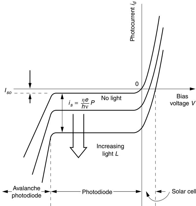
**Figure 16.12** Current–voltage characteristic of a p–n junction.
