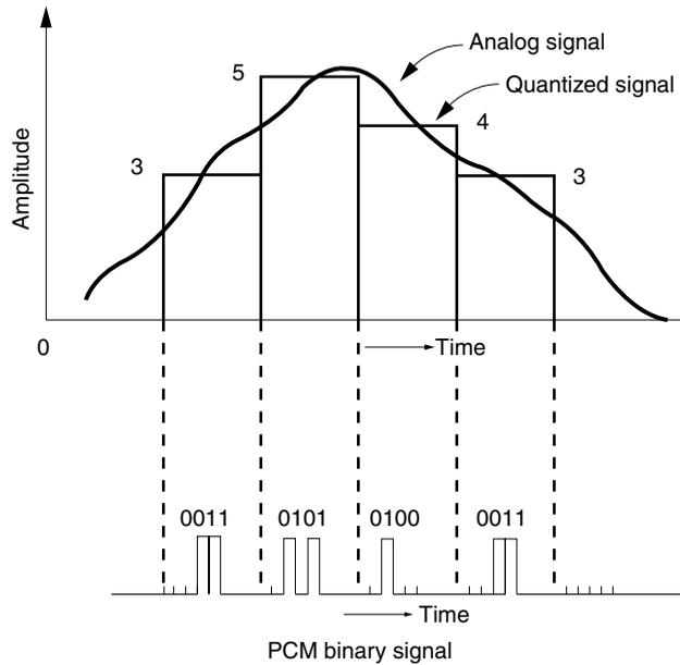
**Figure 16.3** Principle of pulse code modulation (PCM).
