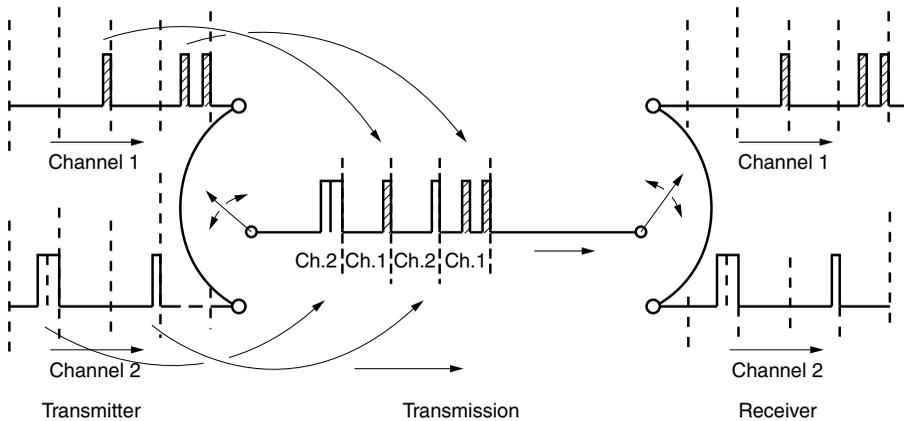
Figure 16.11 Time division multiplexing (TDM) and demultiplexing.
