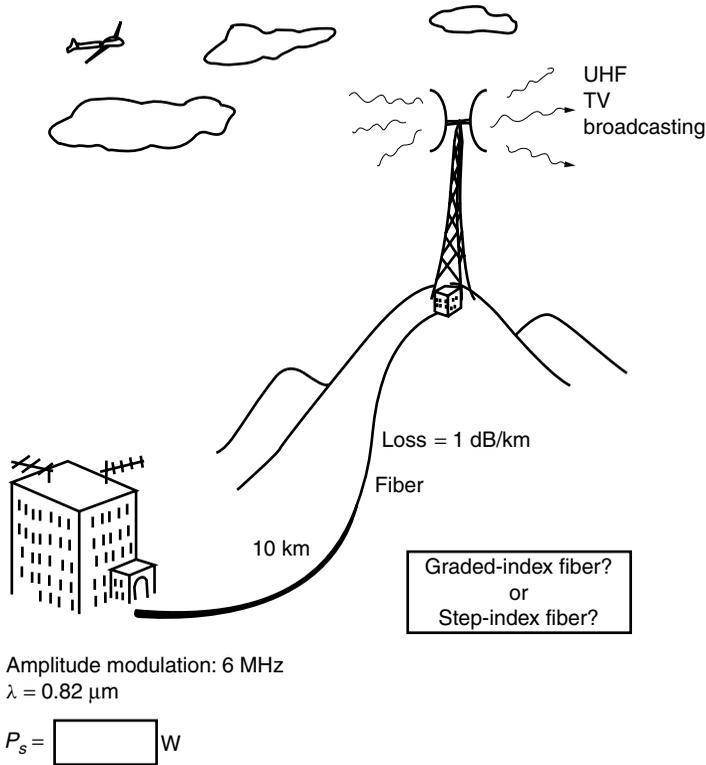
Figure 16.28 Another example of an analog system design.
