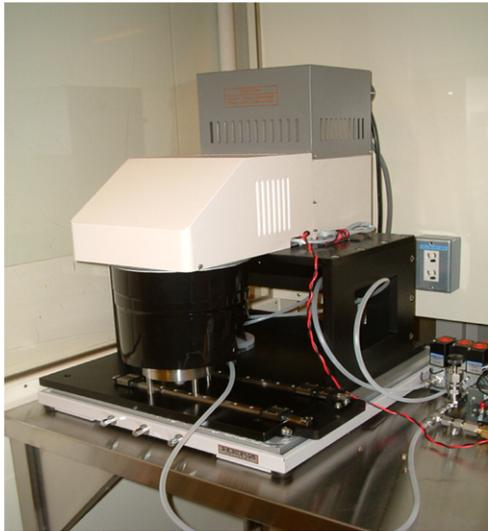
**Fig. 4.3.** Near-field pattern exposure system. The mask is brought into intimate contact with the resist surface, and a g-line light emitted from a mercury lamp is illuminated
