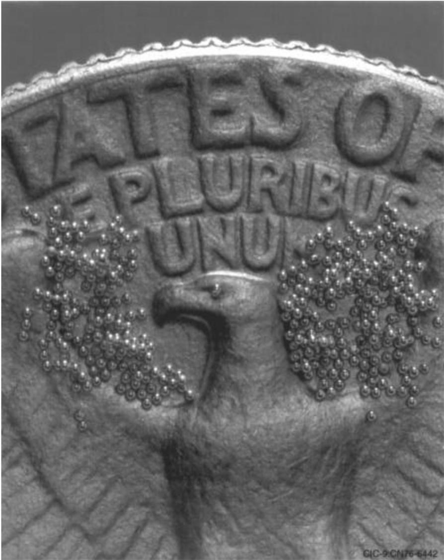
FIG. 14.5 Gold microshells containing high pressure D-T gas for use in laser fusion (Courtesy Los Alamos National Laboratory, No. CN 76-6442).
