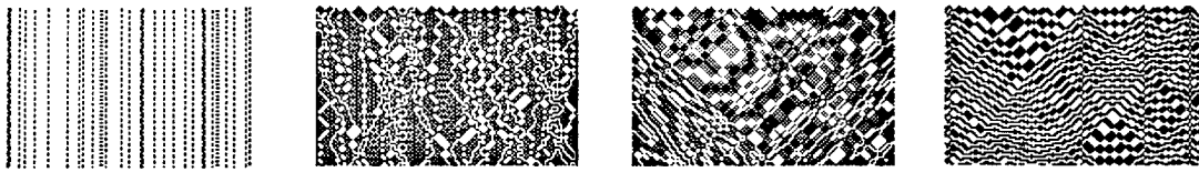
Fig. 7 Evolution of some cellular automata with reversible rules. Each configuration is a unique function of the two previous configurations. (Rule numbers 4, 22, 90 and 126 are shown.) As initial conditions, each site in two successive configurations is chosen to have value 1 with probability 0.1.
