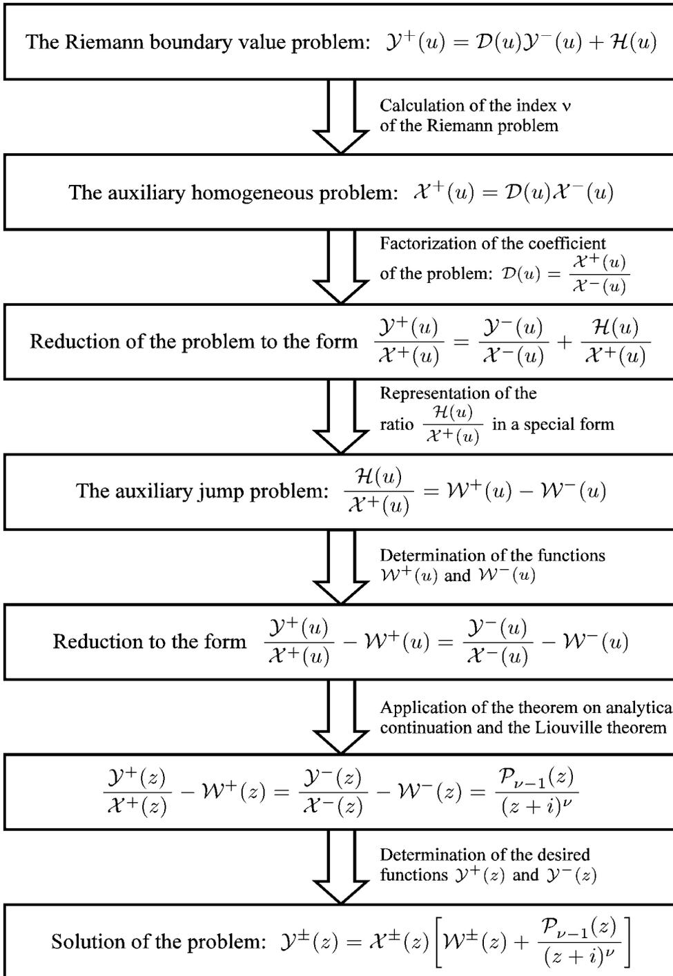
Fig. 3. Scheme of solving the Riemann boundary value problem for the functions  $\mathcal{Y}^+(z)$  and  $\mathcal{Y}^-(z)$  that are analytic, respectively, in the upper and the lower half-plane of the complex plane  $z = u + iv$ . It is assumed that  $\mathcal{D}(u) \neq 0$  and  $\mathcal{P}_{\nu-1}(z) \equiv 0$  for  $\nu \leq 0$ .
