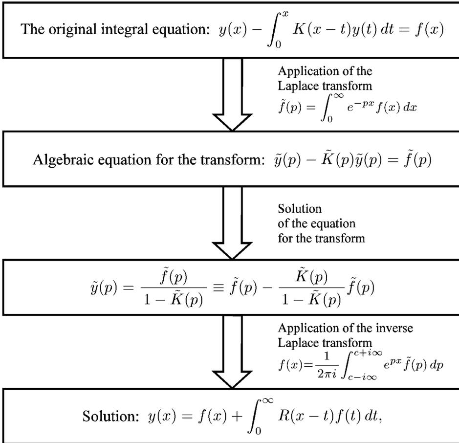
Fig. 2. Scheme of solving Volterra integral equations of the second kind with difference kernel by means of the Laplace integral transform.  $R(x)$  is the inverse transform of the function  $\tilde{R}(p) = \frac{\tilde{K}(p)}{1 - \tilde{K}(p)}$ .
