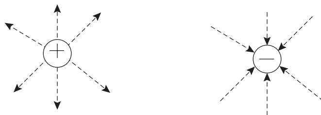
Figure 12.5 Electric field lines produced by point charges.
