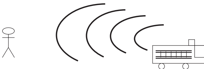
Figure 15.10b As the fire truck moves away from you, the sound waves spread apart, and you hear a lower frequency.
