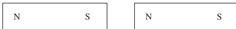
Figure 14.2 Cutting the bar magnet in Figure 14.1 in half just gives you two smaller bar magnets. You can never get an isolated north or south pole.
