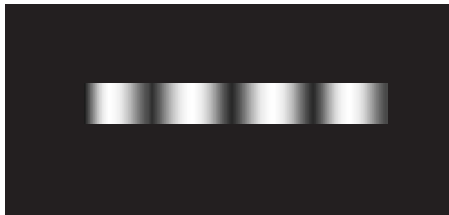
Figure 15.12b Image on the screen in the double-slit experiment.
