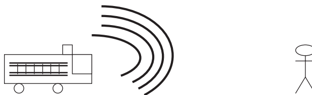
Figure 15.10a When the fire truck moves toward you, the sound waves get squished together, increasing the frequency you hear.
