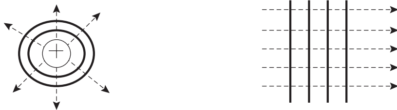
Figure 12.2 Two examples of equipotential lines (in bold) and electric field lines (dotted).
