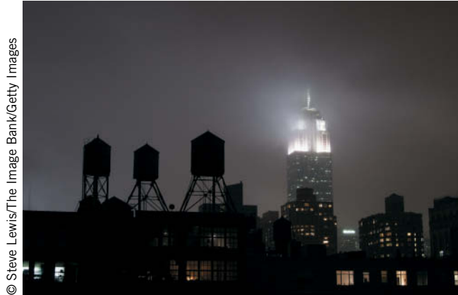
Fig. 5.2.8 Many buildings in New York City have water towers on their roofs. These towers maintain water pressure in the plumbing and help in firefighting.
