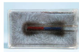
Fig. 11.1.8 Supported by a liquid, this iron powder shows the magnetic flux lines around the magnet.
