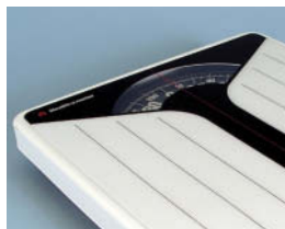
Fig. 3.1.4 When you step on this bathroom scale, its surface moves downward slightly and compresses a stiff spring. The extent of this compression is proportional to your weight, which is reported by the dial. Levers inside the scale make it insensitive to exactly where you stand.
