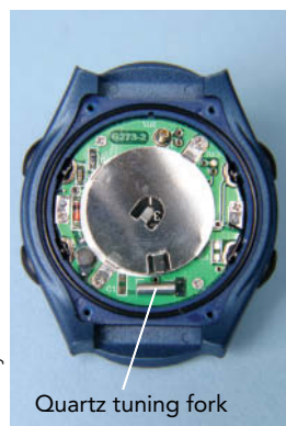
Fig. 9.1.9 The quartz crystal in this wristwatch is located inside the silver cylinder at the bottom. Carefully polished to vibrate at a precise frequency, the crystal keeps the watch accurate to a few seconds a month.
