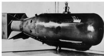
Fig. 15.1.7 The Little Boy (a) used a cannon to fire a cylinder of uranium into an incomplete sphere of uranium. The Fat Man (b) used high explosives to crush a sphere of plutonium to extreme density. Little Boy destroyed Hiroshima, and Fat Man destroyed Nagasaki.
