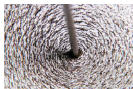
Fig. 11.1.9 Iron powder shows that flux lines around a current-carrying wire form concentric rings around that wire.
