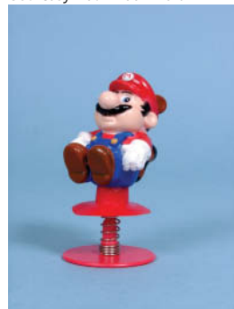
Fig. 15.1.3 This hopping toy stores energy as its spring is compressed and retains that energy while its suction cup grips its base. When the suction cup lets go, the toy leaps into the air.
