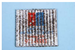
Fig. 11.1.5 Iron powder forms bridges between the magnetic poles of this plastic sheet magnet.
