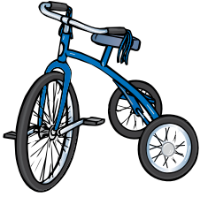
Fig. 4.1.1 A tricycle is very stable when it's standing still. However, it tips over easily during a high-speed turn because the rider can't lean in the direction that the tricycle is turning. The rider must also pedal furiously to move at a reasonable speed.
