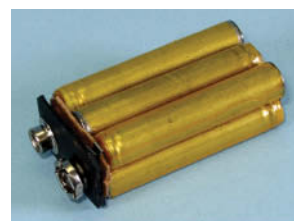
Fig. 10.3.7 A 9-V battery actually contains six small 1.5-V cells, connected in a chain. Positive charges that enter the chain at the battery's negative terminal pass through all six cells before arriving at the battery's positive terminal.
