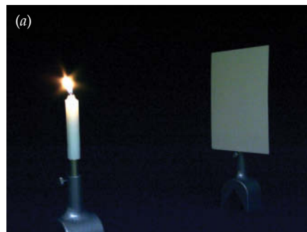
Fig. 14.1.2 (a) When candlelight falls directly on a sheet of paper, it produces no image. (b) A lens inserted between the candle and paper forms an inverted real image of the flame on the paper.
