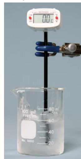
Fig. 7.2.2 Ice and water can coexist only at 0^{\circ}\text{C} , ice's melting temperature.
