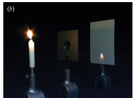
Fig. 14.1.2 (a) When candlelight falls directly on a sheet of paper, it produces no image. (b) A lens inserted between the candle and paper forms an inverted real image of the flame on the paper.
