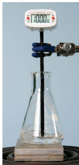
Fig. 7.2.4 Water boils at 100 °C, when atmospheric pressure can no longer smash the bubbles of water vapor.
