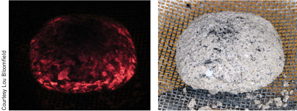
Fig. 7.1.5 A hot charcoal briquette glows brightly in the dark (left). However, a flash photograph reveals that its surface is actually gray and thus a partial absorber of light (right). If it weren't for the white ash, the briquette's black carbon would make it a nearly ideal emitter of blackbody radiation and absorber of light.
