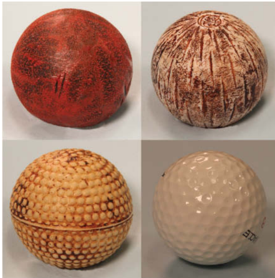
Fig. 6.2.8 Early golf balls were handmade of leather and stuffed with feathers. Golf became popular when cheap balls made of a hard rubber called gutta-percha became available. New, smooth “gutties” (top-left) didn’t travel very far, though; they flew better when they were nicked and worn. Manufacturers soon began to produce balls with various patterns of grooves (top-right) or bumps (bottom-left) on them, and those balls traveled dramatically farther than smooth ones. Modern golf balls (bottom-right) have dimples instead of grooves or bumps.
