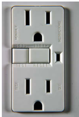
Fig. 11.2.2 This electric outlet follows the U.S. standard for 120-V AC, 15-A service. The wide slots (left) are neutral, the narrow slots (right) are hot, and the curved holes (center) are ground. This outlet provides ground-fault circuit interruption (GFCI) protection; if any current leaving hot fails to return to neutral, or vice versa, the outlet shuts off instantly until it is reset. The test button simulates a current leak and will shut off the outlet if its protection is functioning properly.
