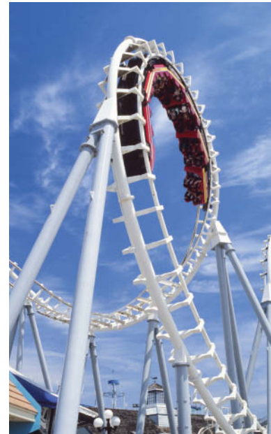
Fig. 3.3.6 As it goes over the loop-the-loop, this roller coaster is accelerating rapidly toward the center of the circle. When it reaches the top of the loop, the track pushes the roller coaster downward and the riders feel pressed into their seats. If they close their eyes, they won't even be able to tell that they're upside down.
