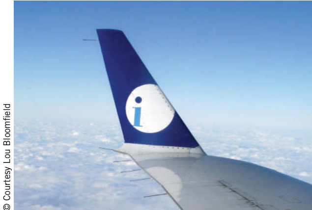
Fig. 6.3.7 This vertical wingtip keeps air from flowing around the end of the wing, a motion that would otherwise leave a powerful vortex in the air trailing behind the plane. Such wingtip vortices waste energy and are hazardous for other aircraft.
