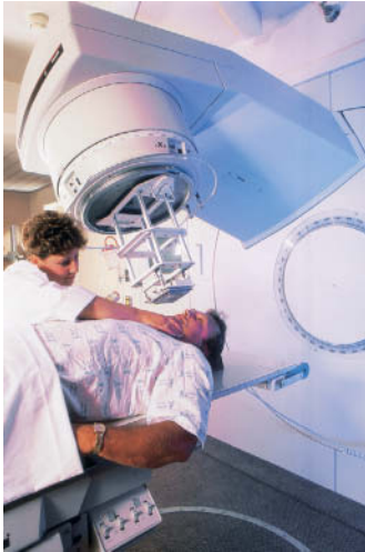
Fig. 15.3.11 This radiation therapy unit uses a linear accelerator to produce extremely high-energy subatomic particles. These particles penetrate deep inside the patient to destroy a cancerous tumor. The linear accelerator itself is hidden from view in the room behind this one. Its beam is steered by magnets in the rotatable arm toward a particular spot in the patient. The arm moves periodically during treatment so that its beam intersects the tumor from many different directions and causes less damage to healthy tissue nearby. That multidirectional strategy is also widely used in X-ray and gamma-ray therapies.
