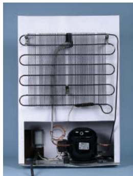
Fig. 8.1.7 The compressor (bottom) and condenser coils (top) are visible on the back of this refrigerator. The compressor squeezes the working fluid into a hot dense gas and delivers it to the condenser. There it gives up heat to the room air and condenses into a liquid. The working fluid evaporates inside the refrigerator, extracting heat from the food.
