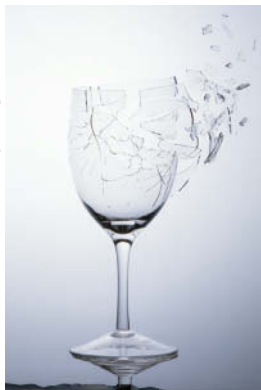
Fig. 9.2.6 Resonant energy transfer makes it possible for sound to shatter a crystal wineglass. When the sound pushes on the glass rhythmically, the sound slowly transfers energy to the glass, until it finally shatters. Because the sound must be extremely loud and at exactly the resonant frequency of the glass, only the most extraordinary opera singers can break a crystal wineglass.
