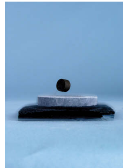
Fig. 11.2.1 A magnetic cylinder floats above the surface of a superconductor at 78 K. Currents flowing freely in the superconductor make it magnetic and cause it to repel the magnetic cylinder.
