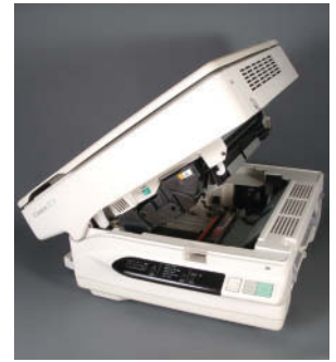
Fig. 10.2.4 This xerographic copier places the photoconductor drum, toner supply, and a corona wire inside a disposable cartridge. After the paper passes through the cartridge, toner is fused onto its surface and it leaves the copier.
