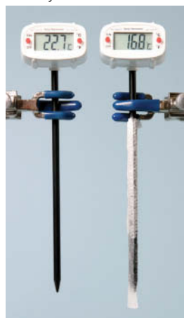
Fig. 7.2.3 You can determine the air's relative humidity using two thermometers, one of which has a wet cloth wrapped around its bulb (right). Evaporation cools the wet-bulb thermometer by an amount related to the air's relative humidity. The dryer the air, the colder the wet-bulb thermometer becomes.
