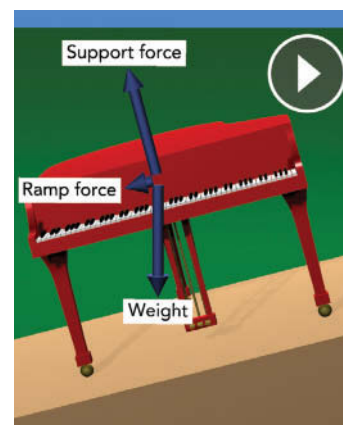
Fig. 1.3.4 When a piano is on a ramp, its weight and the ramp's support force don't cancel. Instead, they sum to a downhill ramp force. If no other forces act on the piano, the ramp force is its net force and it accelerates downhill.
