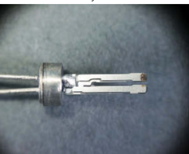
Fig. 9.1.10 Shaped like a tiny tuning fork, this watch crystal vibrates almost exactly 32,768 times per second. Burn marks at its tips were created when its vibrational frequency was tuned by a laser beam.
