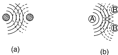
Figure 8.35 Interference between scattered photoelectrons in (a) a gaseous diatomic molecule and (b) a crystalline material
