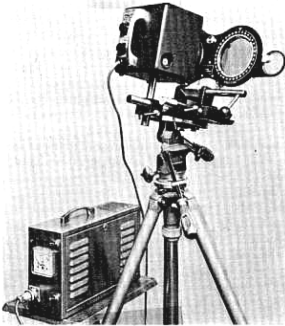
Fig. 6.27. Reflection polariscope principle and equipment.
