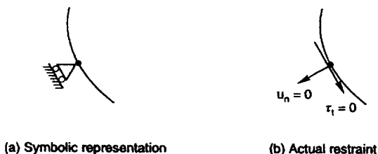
Fig. 9.16. Boundary node with zero shear traction and zero normal displacement.
