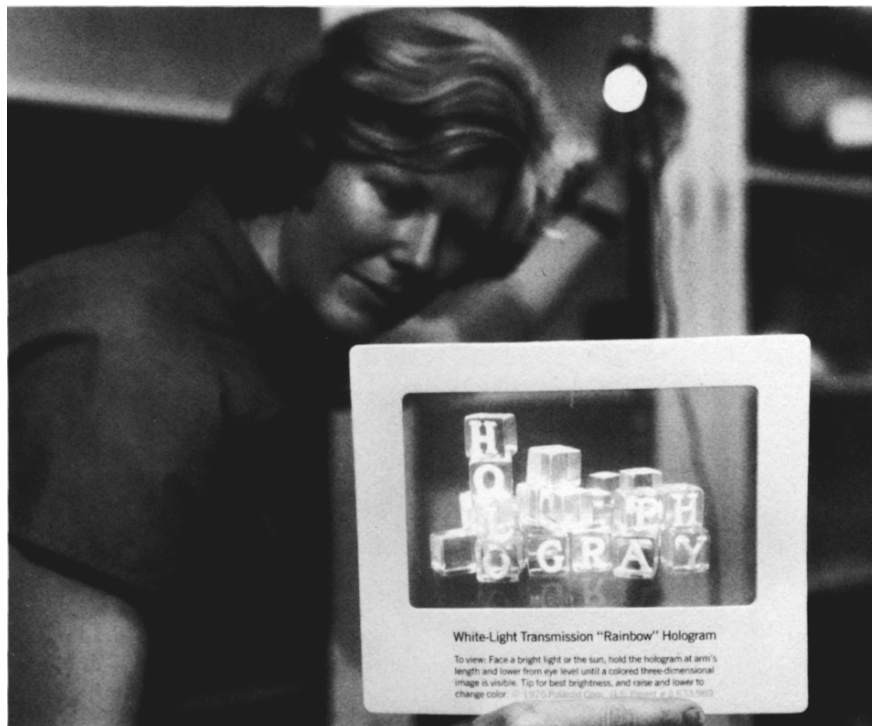
Fig. 8.17 Reconstructed image from the rainbow hologram. The hologram is displayed in an ordinary laboratory environment, showing the high visibility of the image. The illumination source is a small spotlight above and behind the hologram [8.11]
