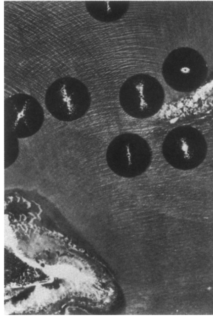
Fig. 11.13 From the Fourier transform of a local region of an aerial picture, the wind direction and magnitude can be decoded [11.7]
