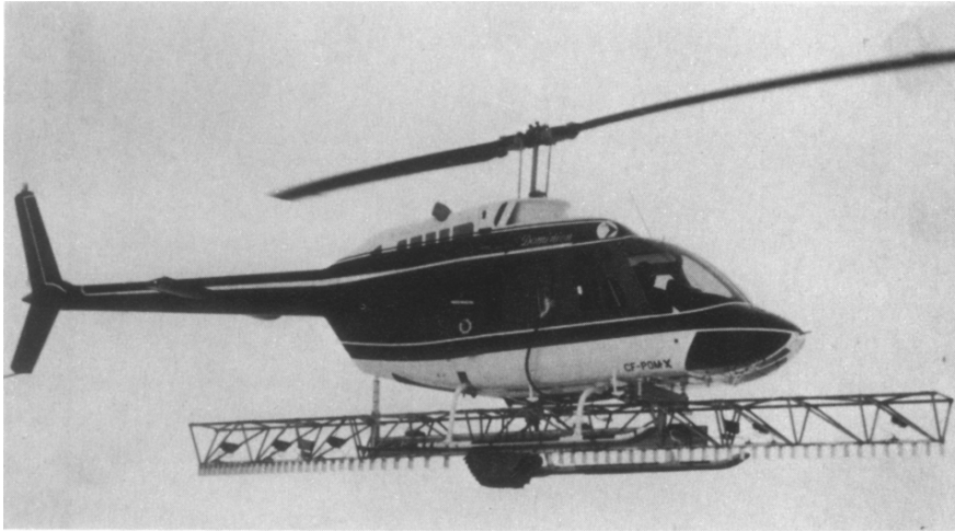
Fig. 12.30 Photograph of HISS radar
