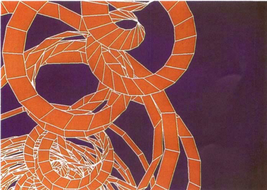
Color Plate 14 Spatially chaotic deformation of the elastica. [From Davies and Moon (1992).]
