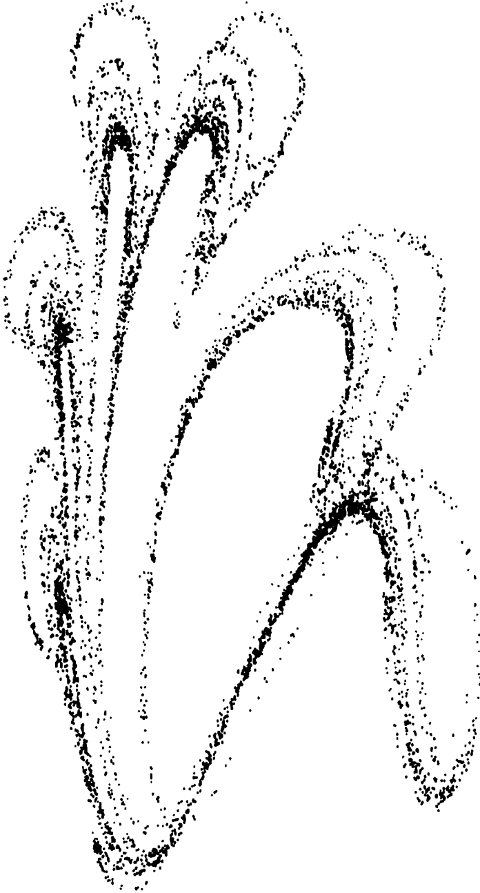
Figure 4-21 Experimental Poincaré map of chaotic motion of the magnetically buckled beam, Fleur de Poincaré.
