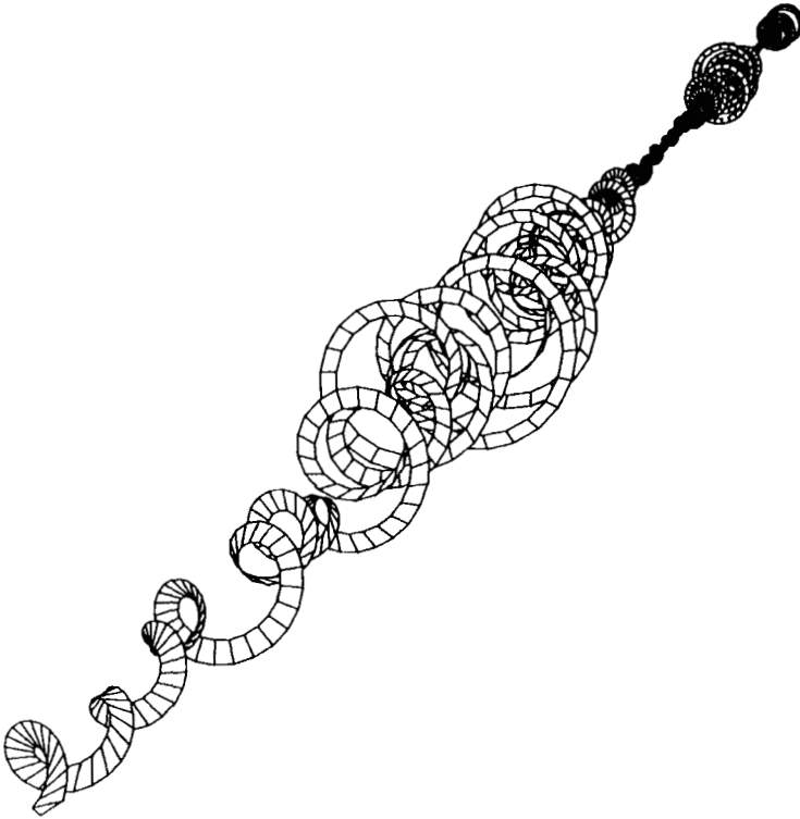
Figure 8-6 Spatial complex twisting deformations of the elastica.
