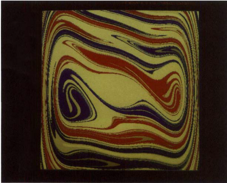
Color Plate 8 Basins of attraction for three-well potential problem in Color Plate 7–force greater than homoclinic criteria. [From Li and Moon (1990a).]
