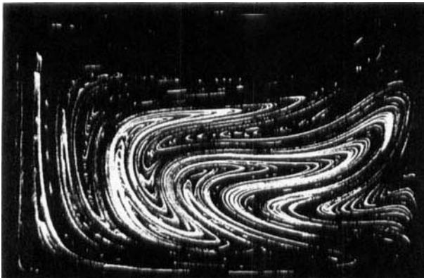
Figure 8-17 Complex mixing patterns for an oscillatory fluid flow process. [From Leong and Ottino (1989).]
