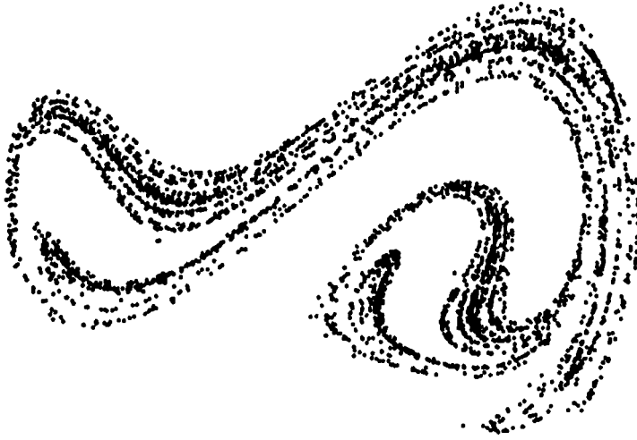
Figure 5-6 Example of an experimental Poincaré map for periodic forcing of a buckled beam.
