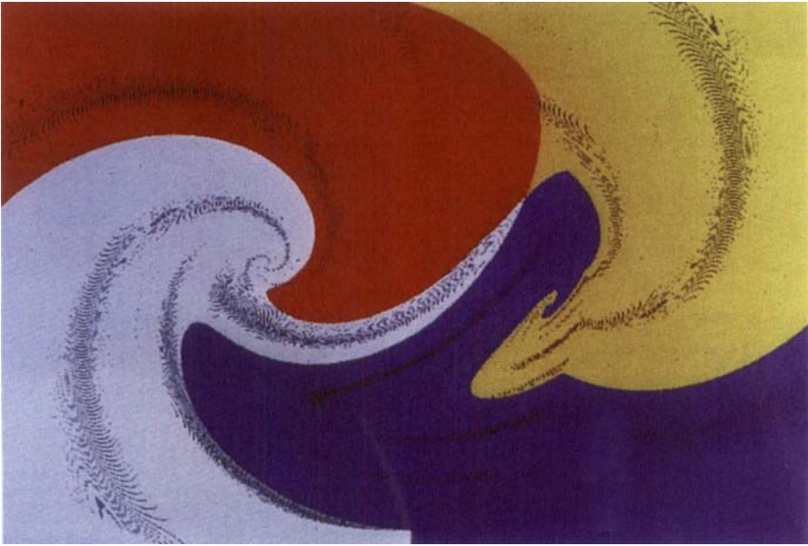
Color Plate 15 Alternating torque mixing of elasto-plastic solids. [From Feeny et al. (1992).]
