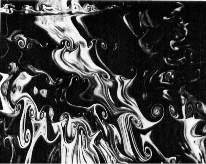
Figure 1-1 Turbulent eddies in the flow of fluid behind a cylinder. (Courtesy of C. Williamson, Cornell University.)
