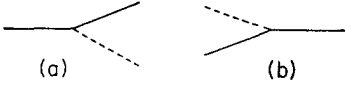
FIG. 6. Diagrams representing the phonon-roton interaction in the Hamiltonian (1'). The solid line is a roton, the broken line a phonon. Time increases from left to right. Diagram (a) represents emission of a phonon, and (b) represents absorption.
