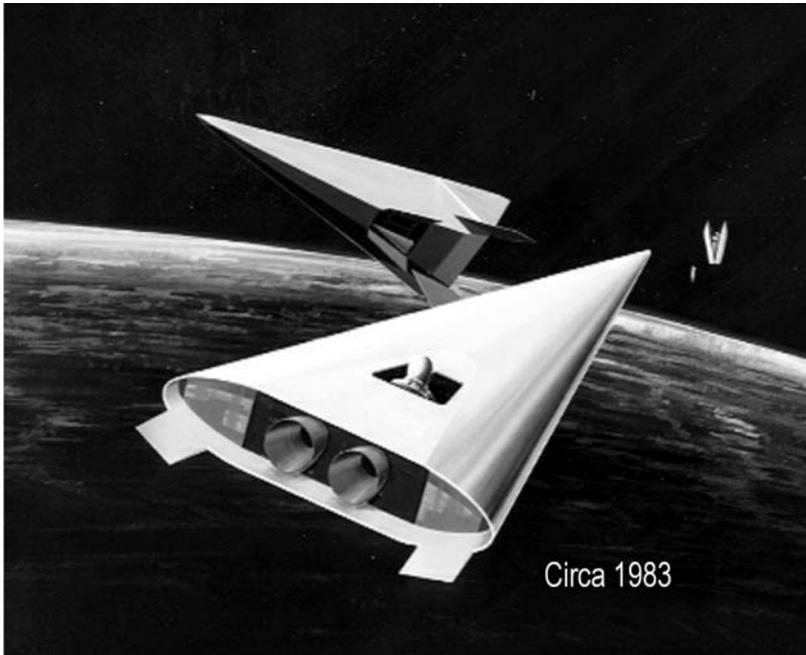
**Figure 2.25.** “Bud” Redding Space Cruiser launched from a trans-atmospheric vehicle to accomplish a satellite repair. The Space Cruiser is able also to serve as a three-person rescue vehicle.
