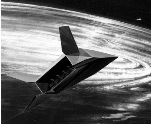
**Figure 5.14.** Aerodynamic turn at 245,000 ft at 22,000 ft/s.
