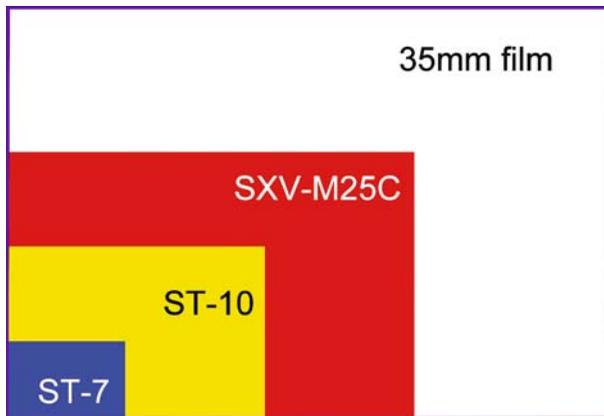
**Figure 2.2.** The relative sizes of the sensors found in some well-known cameras; the SBIG ST-7, the SBIG ST-10 and the Starlight Xpress SXV-M25C. These are compared against the size of film emulsion. Some sensors are now as big as 35 mm film, but they are still rather expensive. Image credit: Grant Privett.
