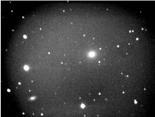
**Figure 3.3.** An example of image vignetting showing the pronounced darkening at the edges and corners of the image. In this example the fall off from full illumination is quite drastic. In other instances it may be a lot more subtle. In all but the most severe cases flat-fielding can help make the whole image usable. Image credit: Gordon Rogers.
