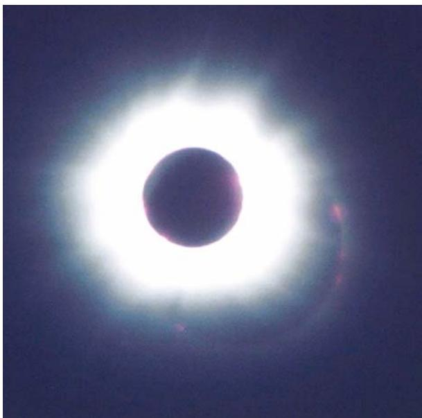
**Figure 3.4.** An example of an internal reflection generated within the optics of a cheap SLR camera. Note how the brightest part of the image – the prominences – form a displaced ring. The contrast has been exaggerated to make it more easily visible. Image credit: Grant Privett.
