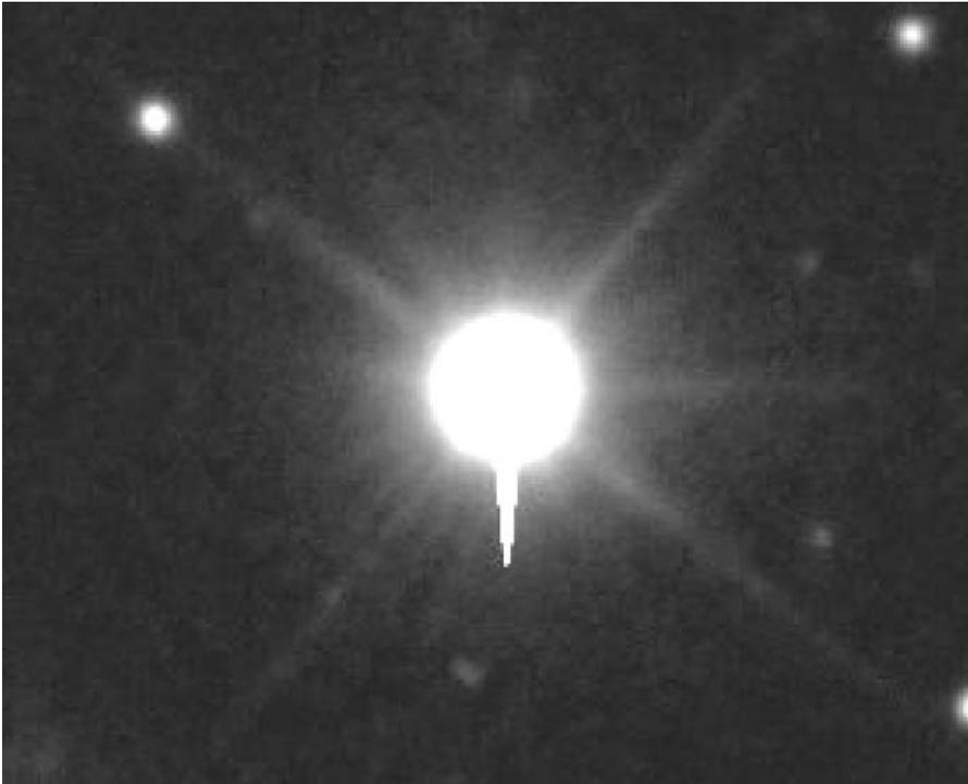
**Figure 8.3.** In this over-exposed star image the four diffraction spikes induced by the spiders supporting secondary mirror can be readily seen. The unsymmetrical spike at the bottom of the star is caused by blooming. Image credit: Gordon Rogers.
