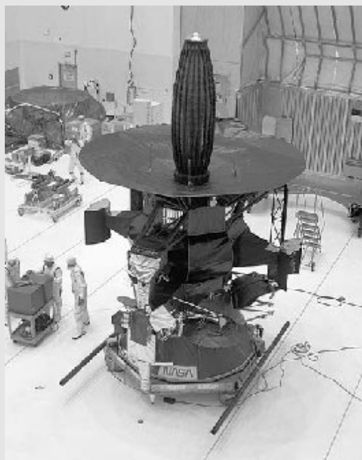
Galileo Galileo being prepared for mating to its Inertial Upper Stage booster at Kennedy Space Center in 1989. NASA
