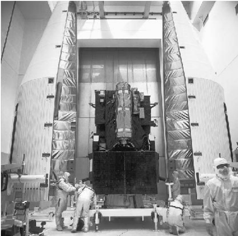
SOHO (Solar and Heliospheric Observatory) SOHO ready to be placed within its protective fairing before transfer to the launch pad. NASA
