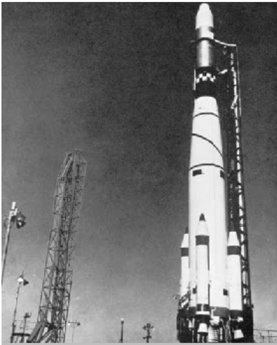
Thor A Thrust Augmented Thor (TAT) Agena D stands on the launch pad. The TAT consisted of a central Thor with four strap-on boosters, which fell away in flight. Douglas Aircraft/Boeing
