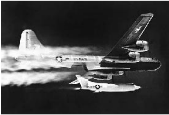
Douglas Skyrocket The Skyrocket begins its flight after dropping from its B-29 mothership. NASA
