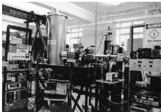
antimatter propulsion An antimatter trap at Pennsylvania State University. Pennsylvania State University
