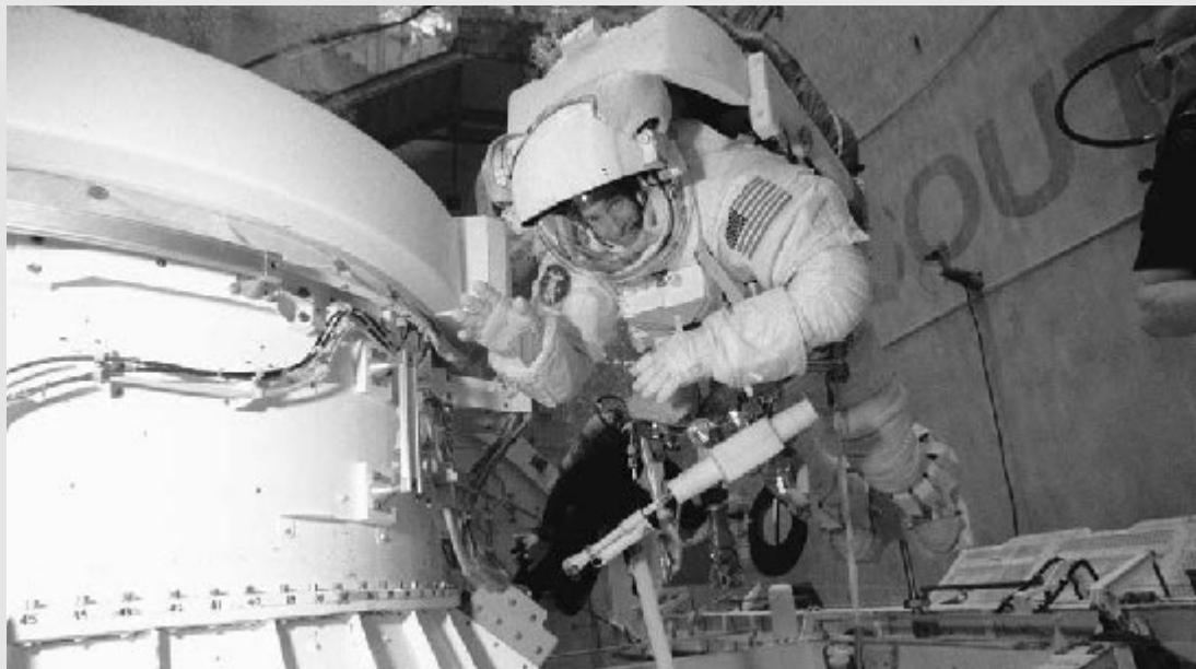
spacesuit Daniel Barry, STS-96 mission specialist, wears a training version of the extravehicular mobility unit spacesuit during an underwater simulation of a spacewalk planned for an early Internal Space Station mission. NASA
