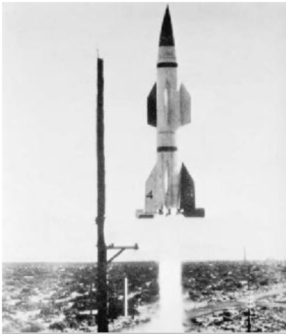
guided missiles, postwar development The first instrumented Hermes A-1 test rocket fired from White Sands Proving Ground. Hermes, based externally on the V-2, contributed to the development of the Redstone missile. NASA
