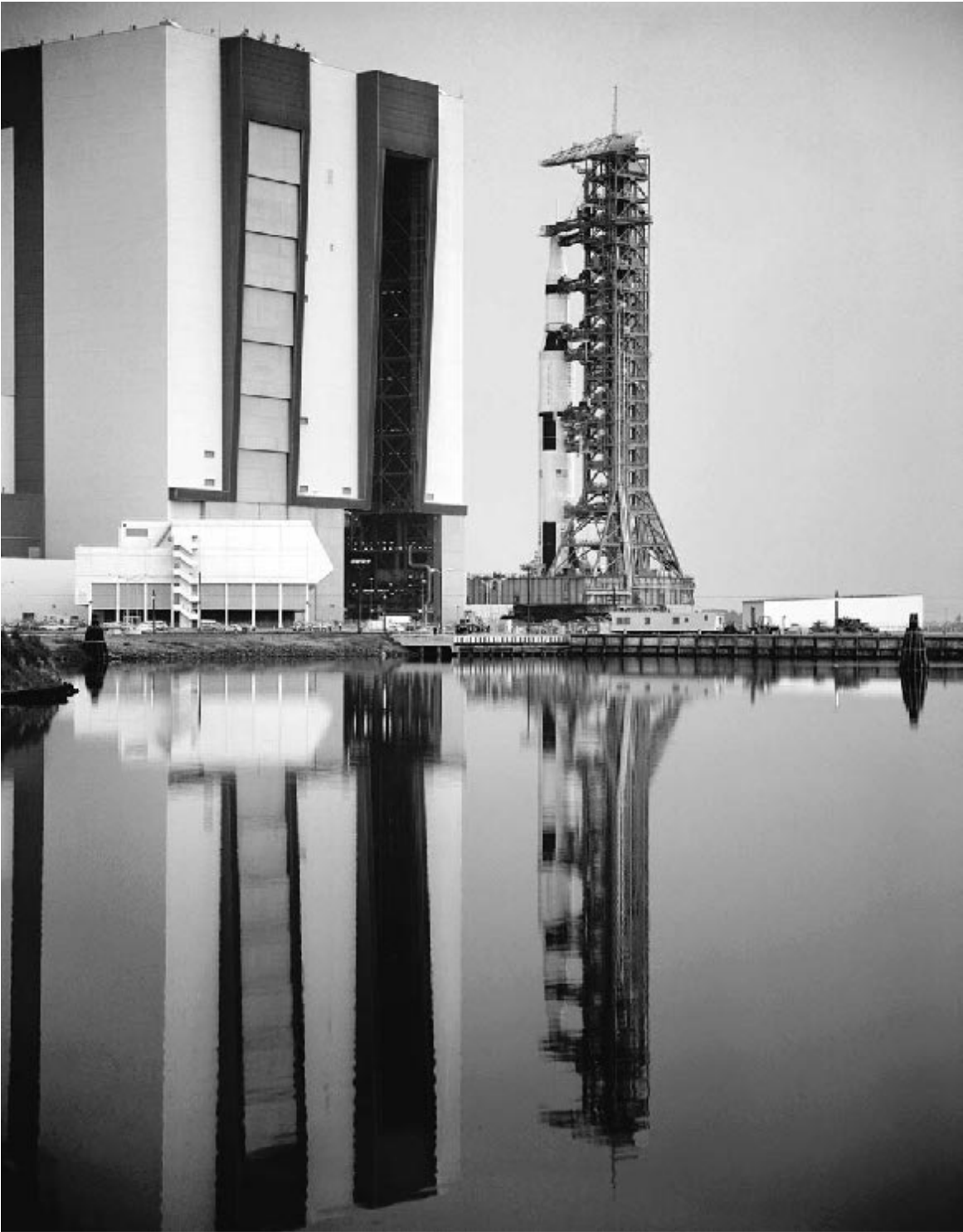
Vehicle Assembly Building The Apollo 15 Saturn V leaving the Vehicle Assembly Building. NASA
