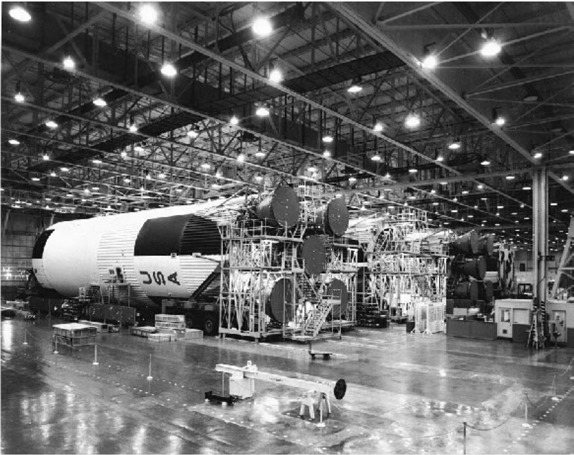
F-1 Five F-1 engines being installed in each of three Saturn V first stages in the horizontal assembly area at NASA's Michoud Assembly Facility. NASA
