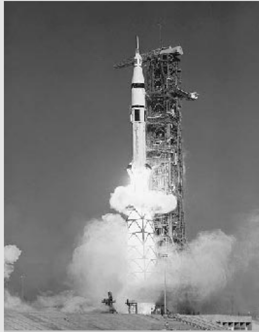
Saturn IB The Saturn IB launch vehicle carrying the Skylab 4 crew lifts off on the final mission to the orbiting space station. NASA
