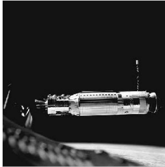
Agena The Agena Target Docking Vehicle, seen from the Gemini 8 spacecraft. NASA
