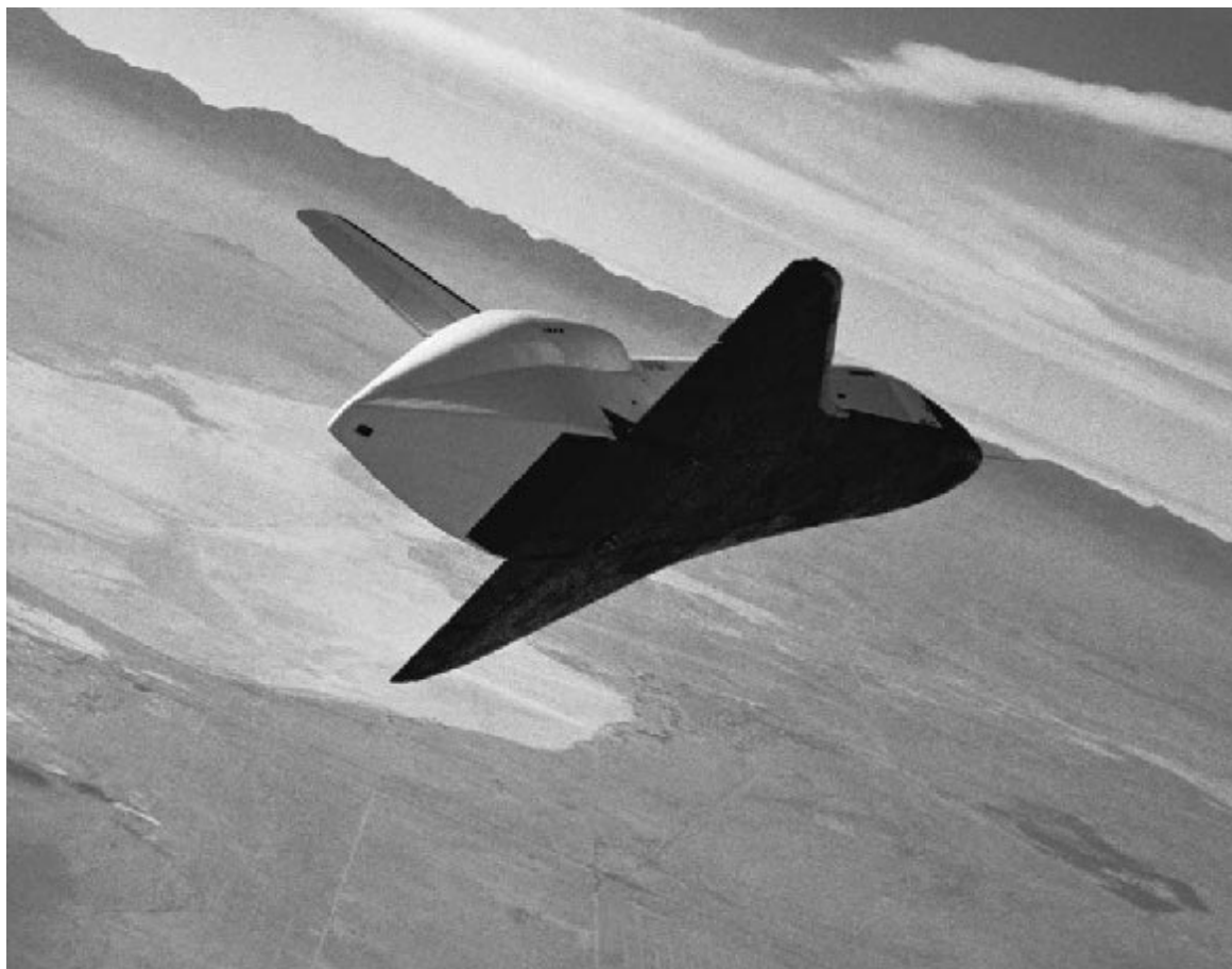
Enterprise Enterprise flies free after being released from NASA's 747 Shuttle Carrier Aircraft over Rogers Dry Lakebed during the second of five free flights carried out as part of the Shuttle program's Approach and Landing Tests. NASA
