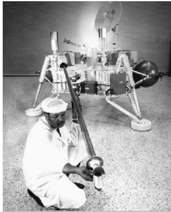
Viking A technician checks the soil sampler of the Viking lander. NASA
