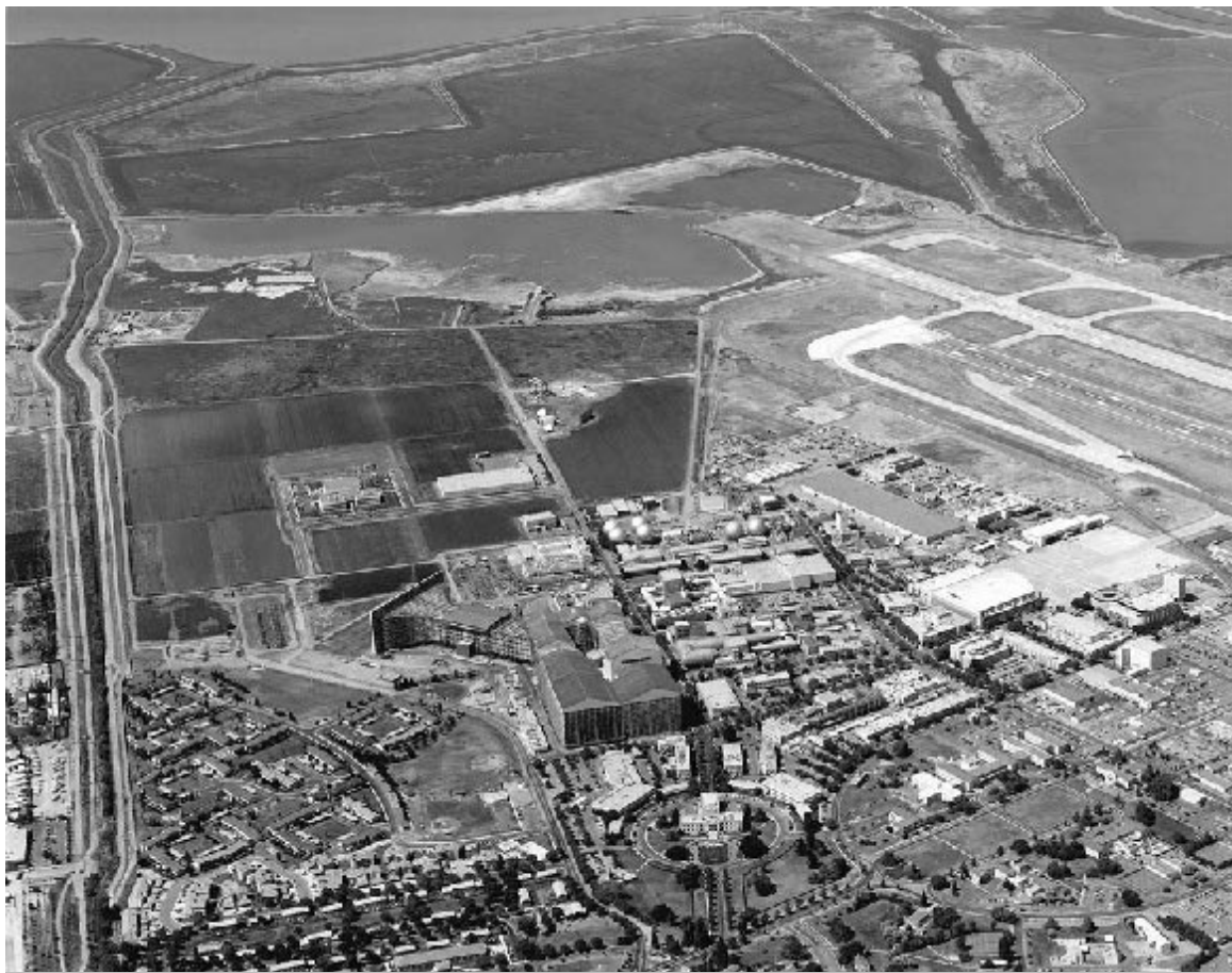
Ames Research Center An aerial view of Ames Research Center. The large flared rectangular structure to the left of center of the photo is the 80 × 120 ft. Full Scale Wind Tunnel. Adjacent to it is the 40 × 80 ft. Full Scale Wind Tunnel, which has been designated a National Historic Landmark. NASA
