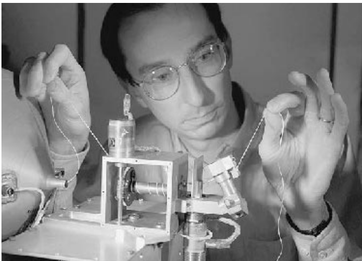
space tether A scientist at the Marshall Space Flight Center inspects the non-conducting part of a tether as it exits a deployer similar to the system to be used in NASA's Propulsive Small Expendable Deployer (ProSEDS) experiment. ProSEDS technology draws power from the space environment around Earth and transfers it to a spacecraft. NASA
