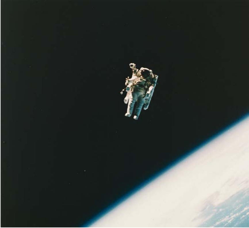
FIG. 8.14 Unprotected from space weather The first untethered walk in space, on 7 February 1984, where there is no place to hide from inclement Sun-driven storms. Astronaut Bruce McCandless II (1937– ), a mission specialist, wears a 300-pound (136-kilogram) Manned Maneuvering Unit (MMU) with 24 nitrogen gas thrusters and a 35 mm camera. The MMU permits motion in space where the sensation of gravity has vanished, but it does not protect the astronaut from solar flares or coronal mass ejections. High-energy particles resulting from these explosions on the Sun could kill the unprotected astronaut. (Courtesy of NASA.)
