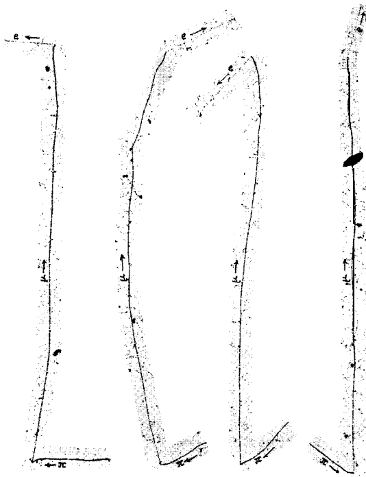
Figure 14.6. Successive decay of the \pi meson, \pi \rightarrow \mu \rightarrow e . (Courtesy P. H. Fowler.)
